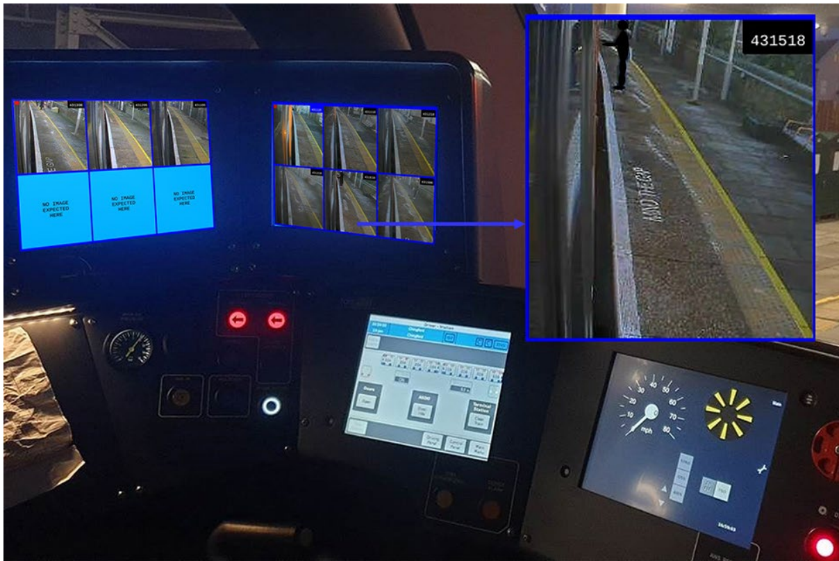
Reconstruction of the driver's in-cab screen using images from the incident CCTV at the moment that door interlock was obtained (the passenger's image has been obscured for publication)
