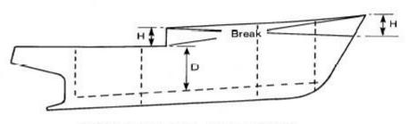
DEPTH OF A VESSEL WITH A BREAK
