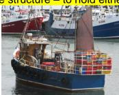
An example of where the catcher is not included is shown below, the catcher is removable, this vessel is used for trawling and creels, with the cat catcher fitted for creels but has to be moved for trawling otherwise the net would foul on its way to the net drum
