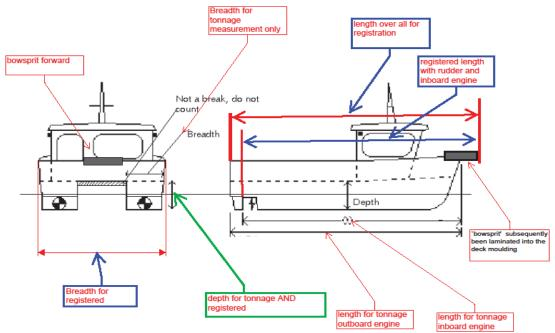
Diagram 2 – Upwardly stepped foredeck NB – This is not a break
