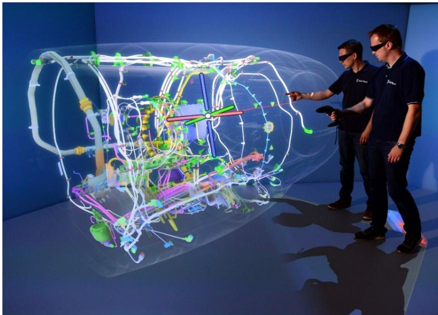
**Figure 6** VR headsets are used to view a digital shadow of a Rolls-Royce jet engine. Copyright: Rolls-Royce
