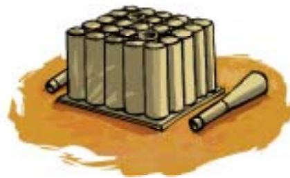
Figure 9.18 TP1 Concrete Substructure cut down to –55m.
