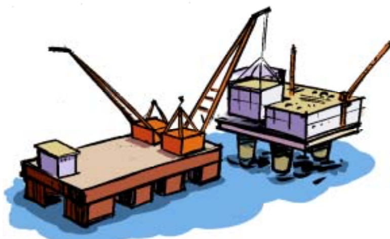
Figure 9.3 Principle of Topsides Removal
