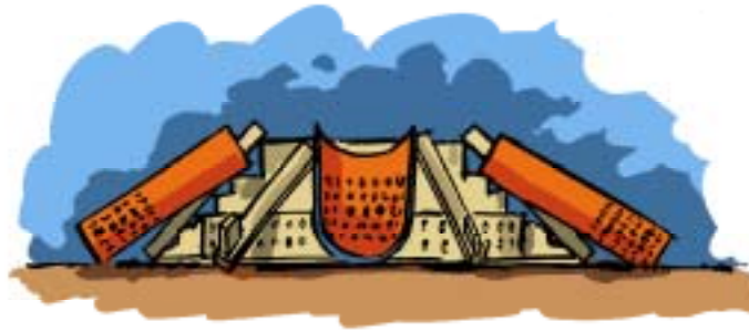
Figure 9.13 CDP1 Concrete Substructure cut down to –55m.
