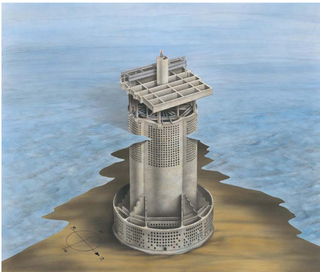
Figure 8.10 Recommended Decommissioned Condition of the MCP-01 Concrete Substructure after Removal of Topside and External Steelwork
