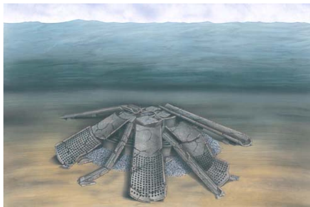
Figure 8.7 MCP-01 Concrete Substructure cut down to –55m.
