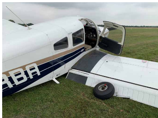
Figure 2 Right wheel assembly and lower portion of the oleo wedged on the flap
