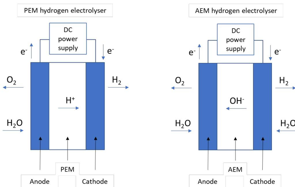
**Figure 2: Schematic of a PEM and AEM (or Alkaline) electrolyser cells showing the hydrogen ions (PEM) and hydroxide anions (AEM) moving between the electrodes. In both cases, electrons are then transported from the anode to the cathode via the electrical circuit.**
