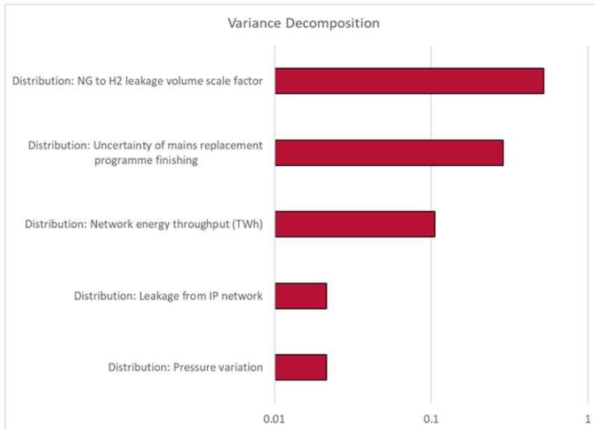
**Figure 14: Variance decomposition of hydrogen transportation in distribution network. The conversation factor from natural gas to hydrogen leakage (based on the gas characteristics and leakage paths in the pipework) is the largest single contributor to uncertainty in the distribution network leakage predictions.**
