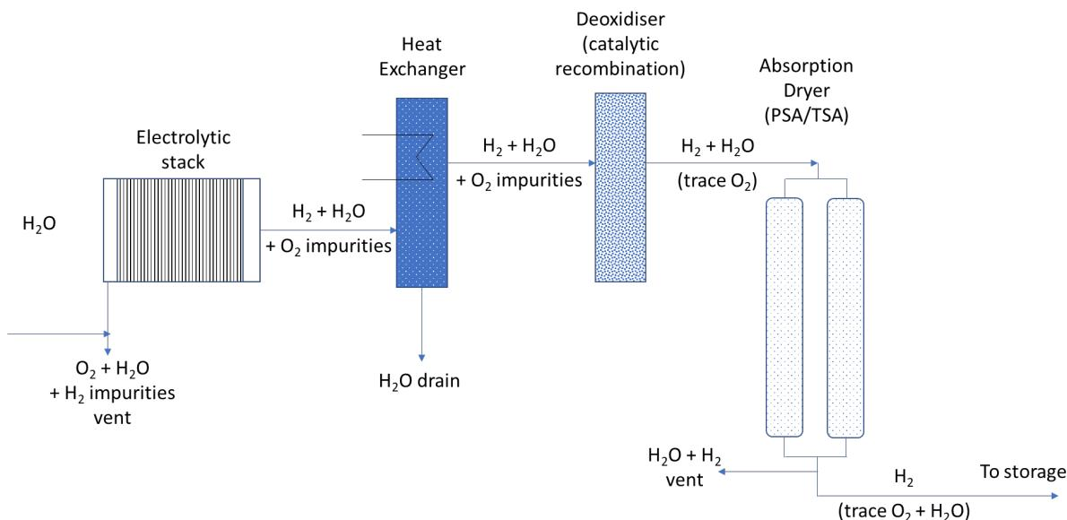
**Figure 4: Schematic of a hydrogen electrolyser system (adapted from [10], [11]).** The hydrogen exiting the electrolysis stack contains water and oxygen impurities. This is passed through a heat exchanger, deoxidiser (catalytic recombiner) and an adsorption dryer (typically Pressure Swing Adsorption (PSA) or Temperature Swing Adsorption (TSA)) to purify the hydrogen.
