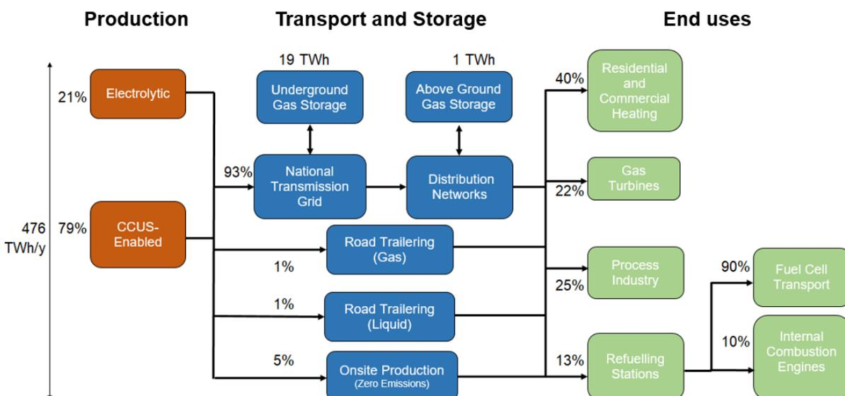
**Figure 1: Schematic of the Central Scenario. The total energy throughput is 476 TWh and the contribution of each element is given as a percentage.**
