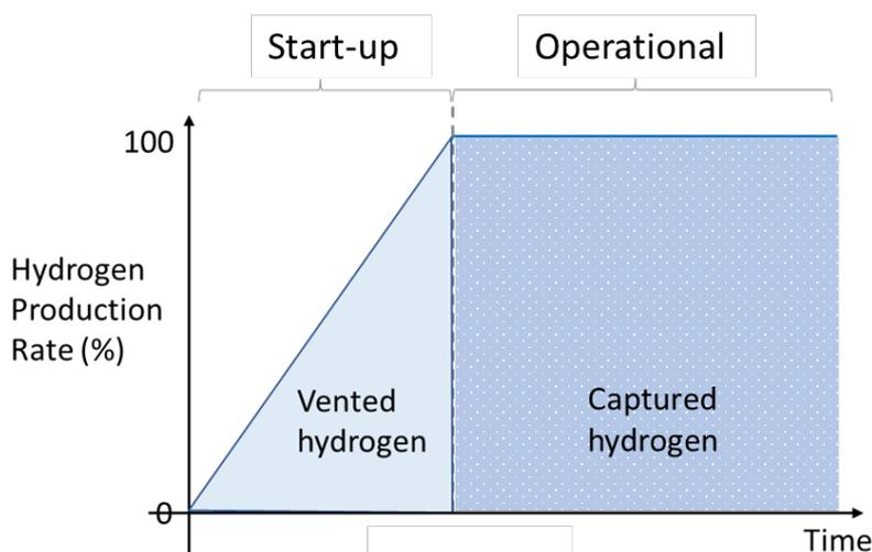
**Figure 3: During the start-up (and shutdown) phases, hydrogen is vented. It is assumed that these follow a linear increase (or decrease) in hydrogen output.**
