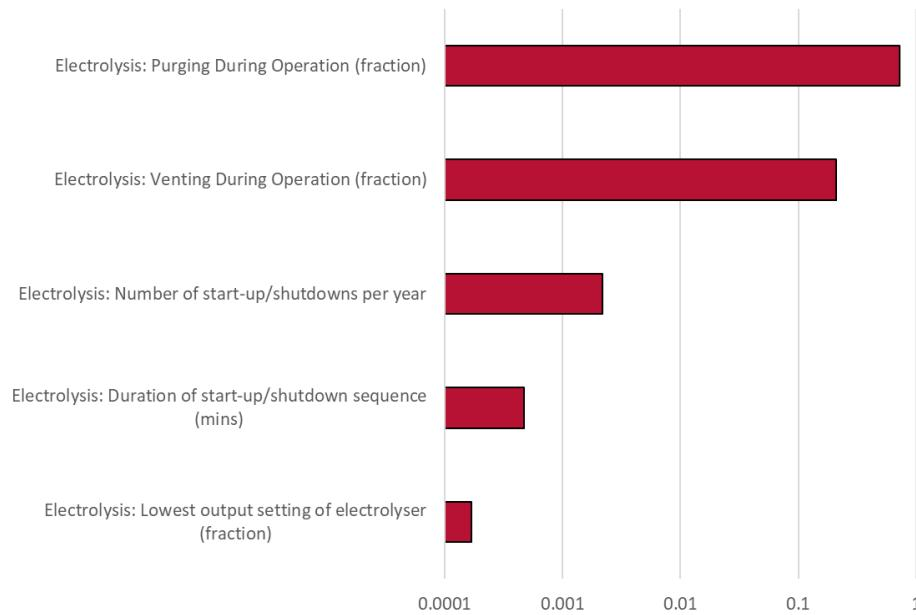
**Figure 9: Variance decomposition of electrolytic hydrogen production. Purging during operation is the single largest contributor to the uncertainty in electrolytic hydrogen emissions, followed by venting during operation.**
