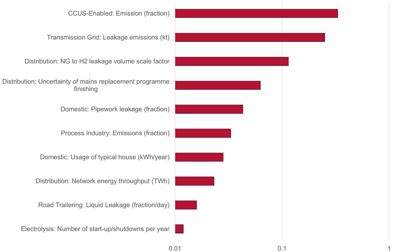
**Figure 12: Variance decomposition for the central scenario. The emissions from CCUS-enabled hydrogen production and the NTS leakage are the largest contributors to the uncertainty in the overall leakage predictions for the central scenario.**
