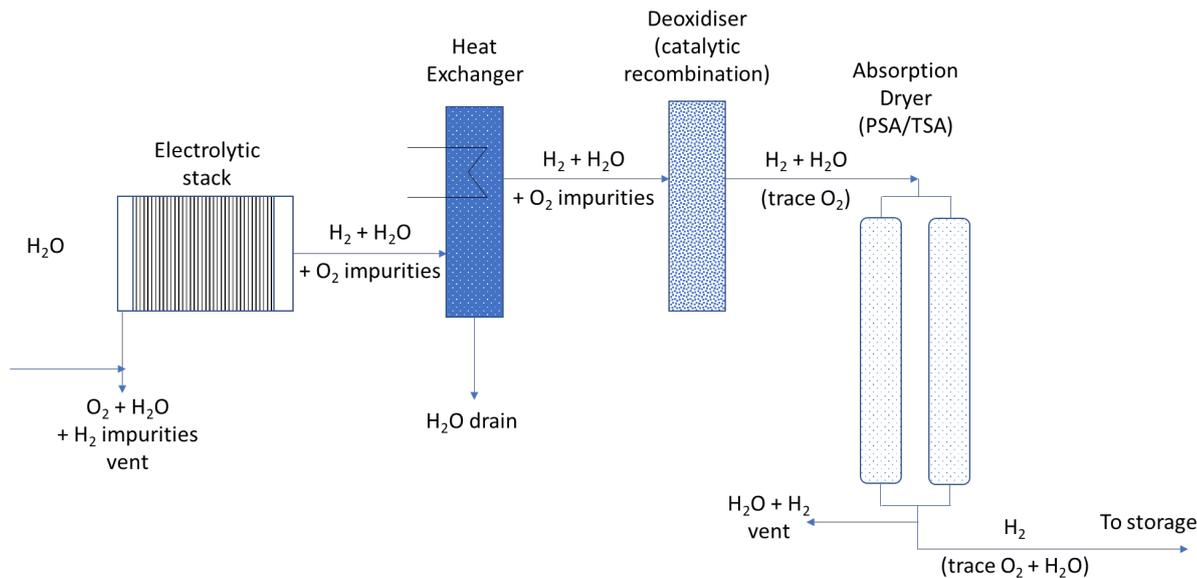
**Figure 4: Schematic of a hydrogen electrolyser system (adapted from [10], [11]). The hydrogen exiting the electrolysis stack contains water and oxygen impurities. This is passed through a heat exchanger, deoxidiser (catalytic recombiner) and an adsorption dryer (typically Pressure Swing Adsorption (PSA) or Temperature Swing Adsorption (TSA)) to purify the hydrogen.**
