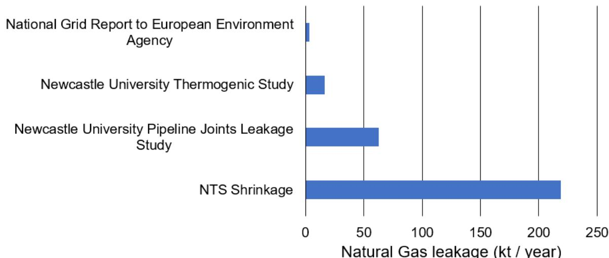
**Figure 5: Comparison of NTS natural gas leakage predictions.** Methane emissions of 3.4 kt/year are reported to the EU, although studies by Newcastle University predict emissions of between 17 (thermogenic emissions only) and 63 kt/year. Shrinkage data obtained from meter readings is much higher at over 200 kt/year but this is considered to be an overestimate.
