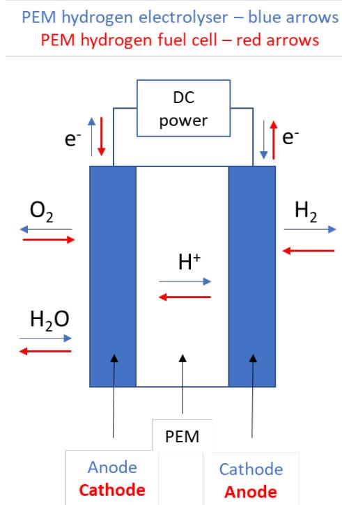
**Figure 7: Difference in operation between a PEM fuel cell and PEM electrolyser. Fuel cells essentially operate as electrolyzers in reverse; the blue lines indicate electrolysis and red lines operating as a fuel cell.**
