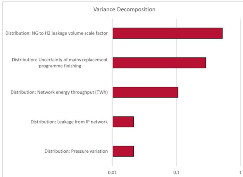
**Figure 14: Variance decomposition of hydrogen transportation in distribution network.** The conversion factor from natural gas to hydrogen leakage (based on the gas characteristics and leakage paths in the pipework) is the largest single contributor to uncertainty in the distribution network leakage predictions.
