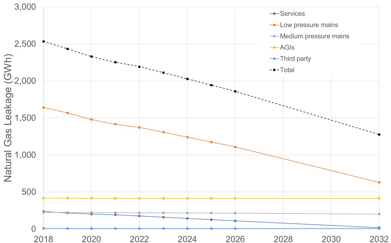
**Figure 6: Gas distribution network leakage predictions up to 2032 provided by OFGEM [22]. By the end of the mains replacement programme in 2032 natural gas leakage is predicted to be 1,277 GWh per year, a 50% reduction since 2018. By 2032, leakage from the low pressure mains will be only slightly higher than from Above Ground Installations (AGI).**
