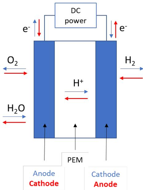
**Figure 7: Difference in operation between a PEM fuel cell and PEM electrolyser. Fuel cells essentially operate as electrolysers in reverse; the blue lines indicate electrolysis and red lines operating as a fuel cell.**
