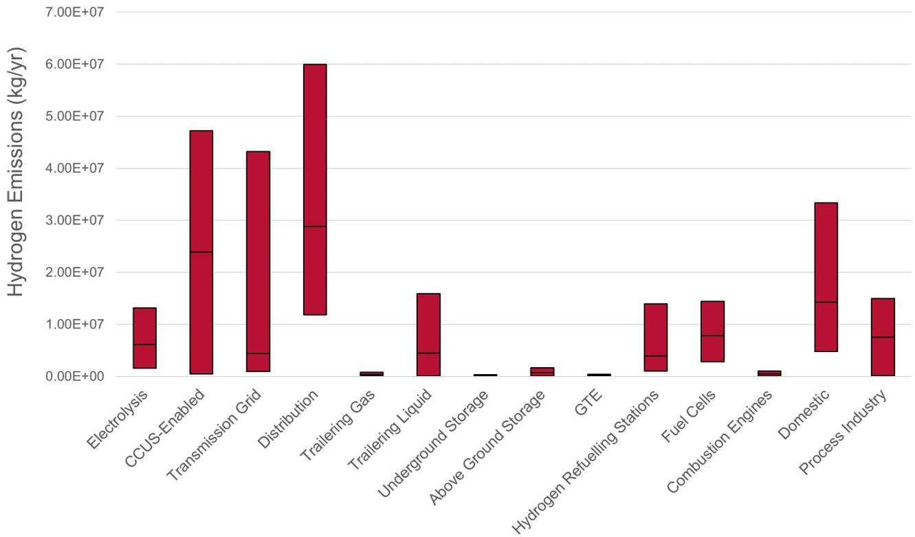
**Figure 11: Central scenario emissions breakdown into individual areas. The bars represent the 1st, 50th and 99th percentiles. The distribution network is predicted to be the element with the single highest hydrogen emissions.**
