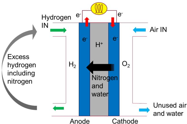
**Figure 8: Schematic of crossover in a fuel cell operation. An excess of hydrogen is supplied to the anode side, which is then recirculated back to the hydrogen inlet.**
