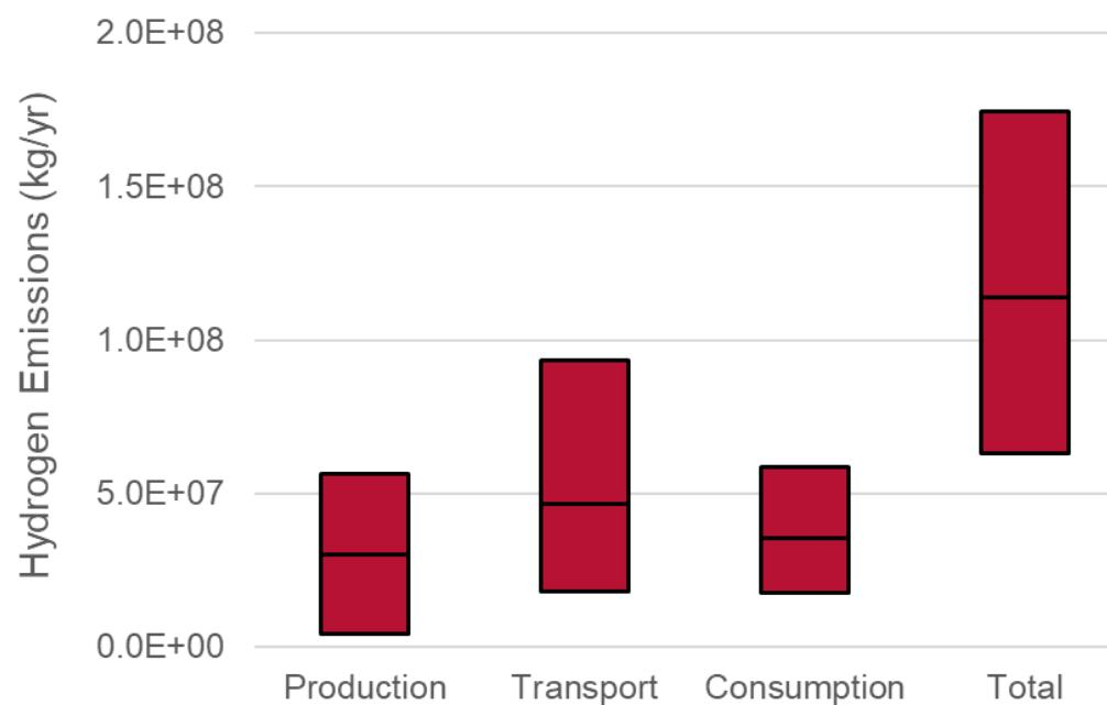
**Figure 10: Central scenario emissions breakdown for production, transport and storage, and consumption. The bars represent the 1<sup>st</sup>, 50<sup>th</sup> and 99<sup>th</sup> percentiles (confidence levels). Transport and storage is predicted to have the largest hydrogen emissions out of the three sectors (production, transport and storage, consumption)**
