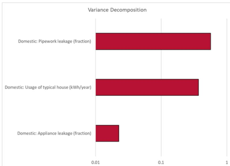
**Figure 15: Variance decomposition of hydrogen transportation in domestic heating. The leakage from domestic pipework is the largest single contributor to the leakage predictions for domestic and commercial heating with 100% hydrogen.**
