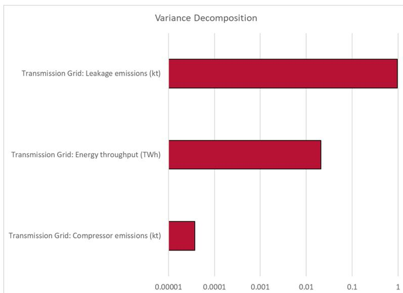
**Figure 13: Variance decomposition of hydrogen transportation in the NTS. The single largest contributor to uncertainty in leakage predictions of a future 100% hydrogen NTS is the extent to which the existing NTS would leak if it was converted to transport 100% hydrogen.**
