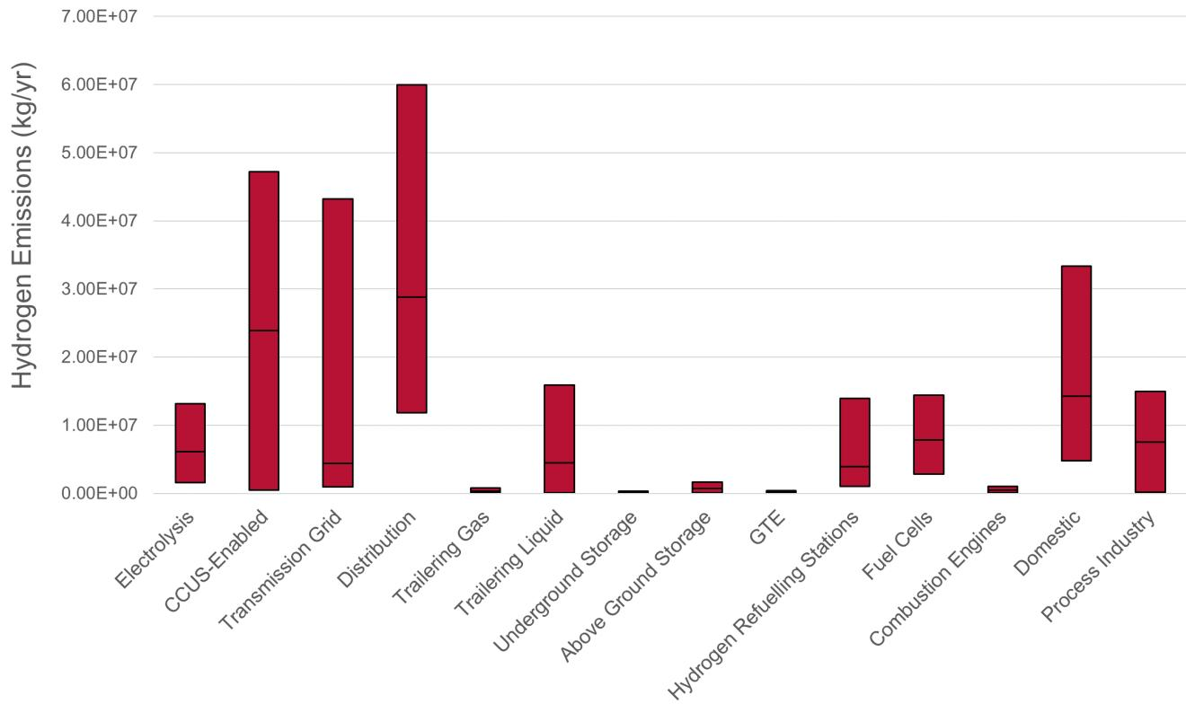
**Figure 11: Central scenario emissions breakdown into individual areas. The bars represent the 1st, 50th and 99th percentiles. The distribution network is predicted to be the element with the single highest hydrogen emissions.**
