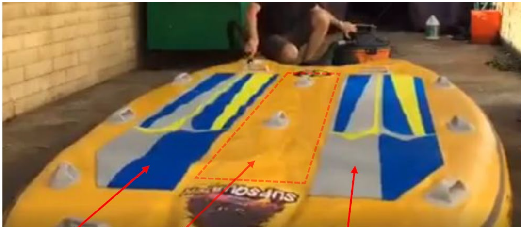
Figure 1.4 - Supsquatch unrolled and being inflated. The red marquee shows the longitudinal gap between the two deck pads
