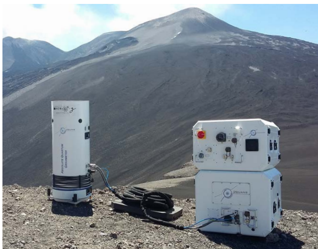
Field-compatible Absolute Quantum Gravimeter developed by Muquans. This picture was taken on Mount Etna volcano as part of the H2020 project Newton-g.
