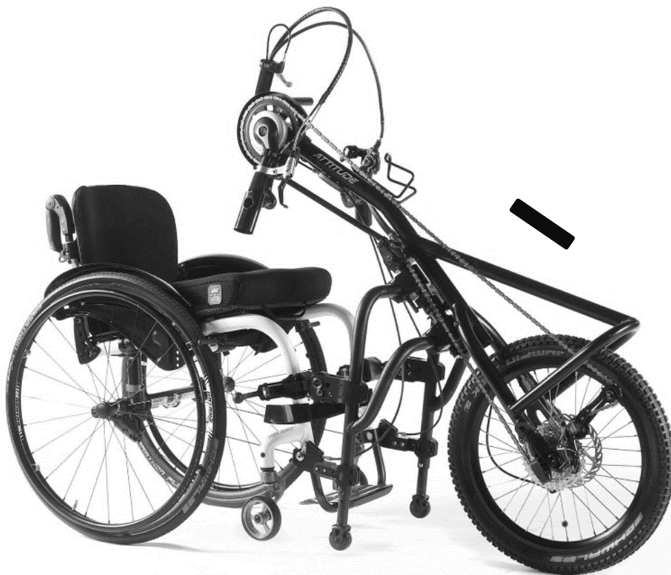
Figure 4.16 Example Hybrid Mobility Aid – Wheelchair with Hand Cycle Attachment
