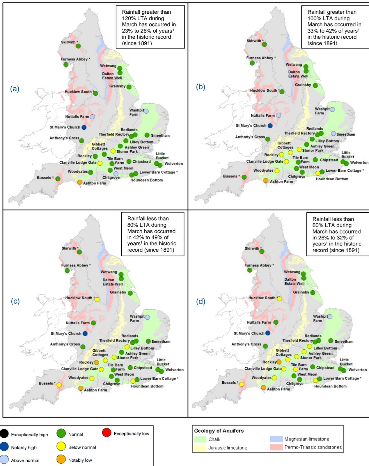
**Figure 6.5:** Projected groundwater levels at key indicator sites at the end of March 2022. Projections based on four scenarios: 120% (a), 100% (b), 80% (c) and 60% (d) of long term average rainfall in March 2022 (Source: Environment Agency) Geological map reproduced with kind permission from UK Groundwater Forum BGS © NERC. Crown copyright all rights reserved. Environment Agency 10024198, 2022.
