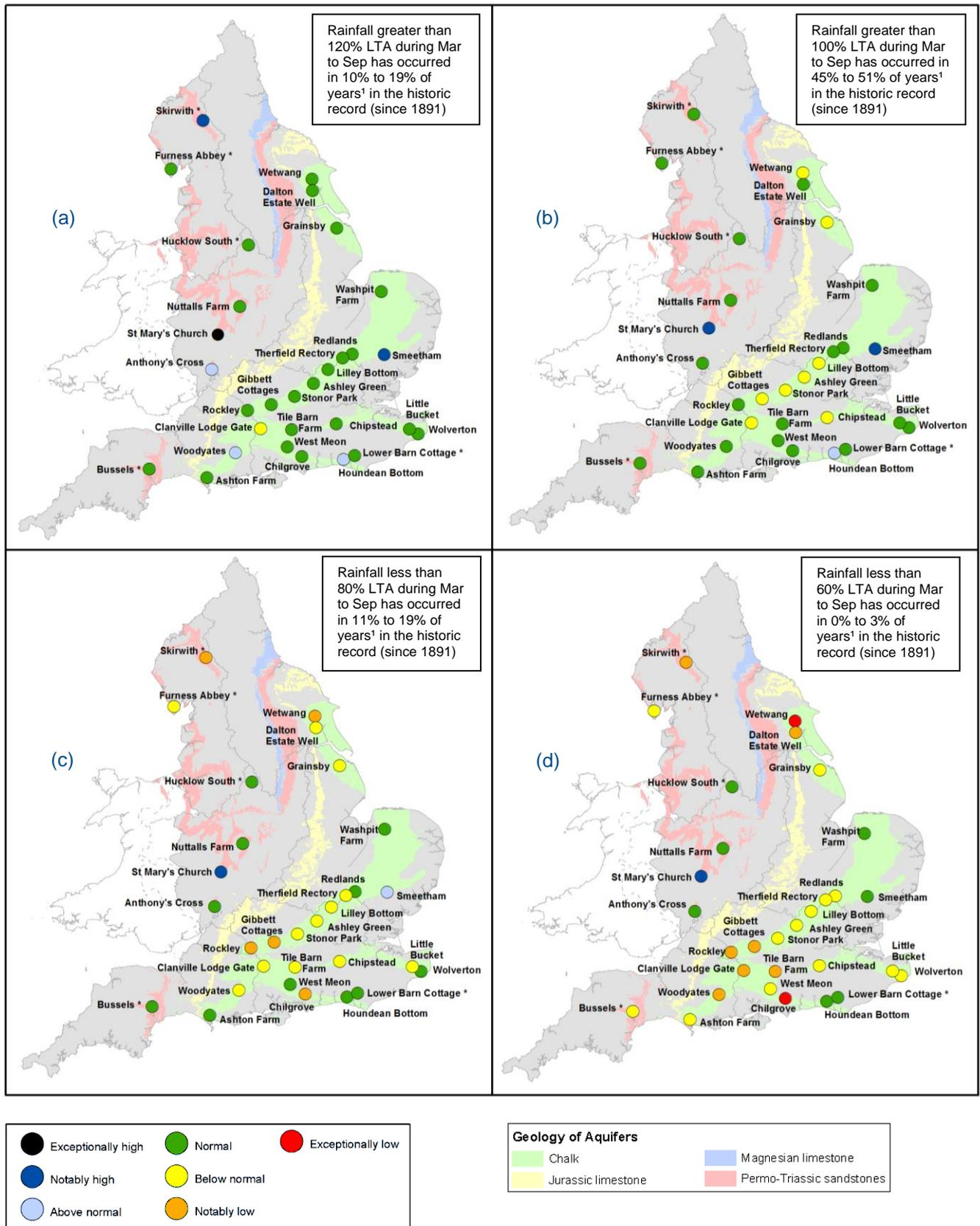
**Figure 6.6:** Projected groundwater levels at key indicator sites at the end of September 2022. Projections based on four scenarios: 120% (a), 100% (b), 80% (c) and 60% (d) of long term average rainfall between March 2022 and September 2022 (Source: Environment Agency) Geological map reproduced with kind permission from UK Groundwater Forum BGS © NERC Crown copyright. All rights reserved. Environment Agency 100024198 2022.
