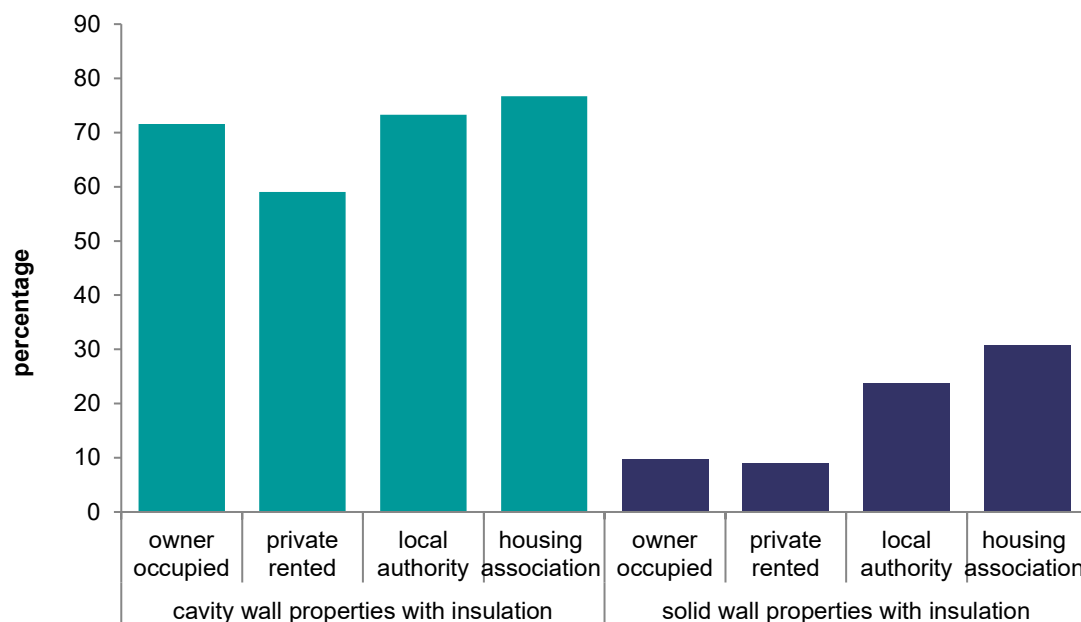
Figure 2.14: Wall insulation, by main wall type and tenure, 2020
