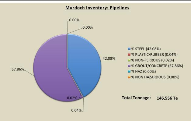
Figure 2.8.2: Pie-chart of estimated pipeline inventory, excl. deposited rock
