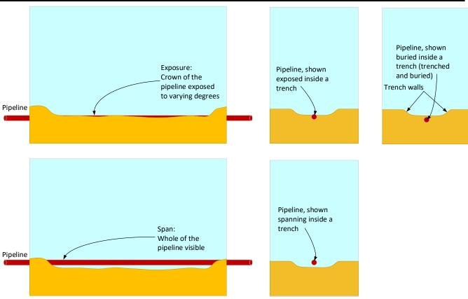
Figure 1.1.1: The difference between pipeline burial, exposures, and spans<sup>1</sup>
