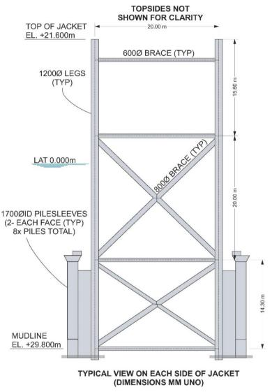
Figure 3.2.3: Murdoch MD jacket typical side view
