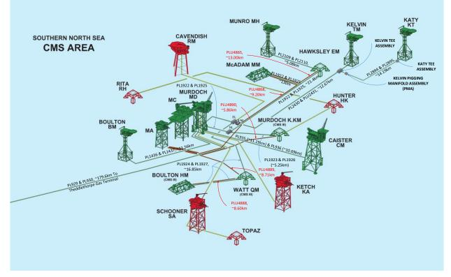
Figure 1.3.1: Murdoch and CMS Area Installations and Pipelines
