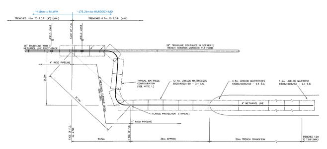
Figure 2.6.4: Separation of PL930 & PL929 ~4.8km from MLWM (NTS)
