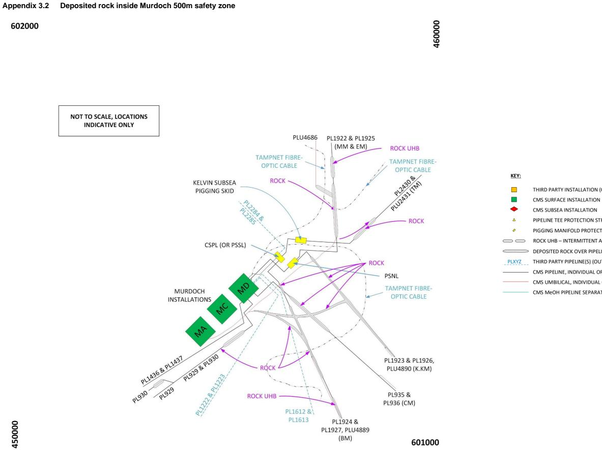
Figure A3.2.1: Schematic of deposited rock inside Murdoch 500m zone
