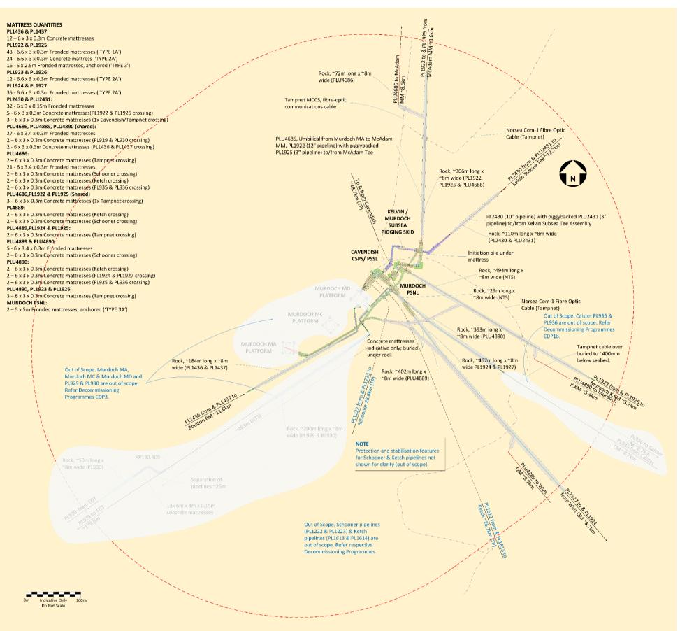
Figure A1.1.1: Schematic of pipelines near Murdoch installations
