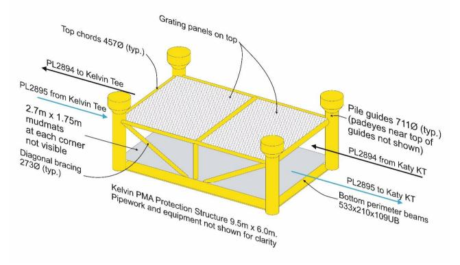
Figure 2.3.3: Perspective of the Kelvin PMA protection structure
