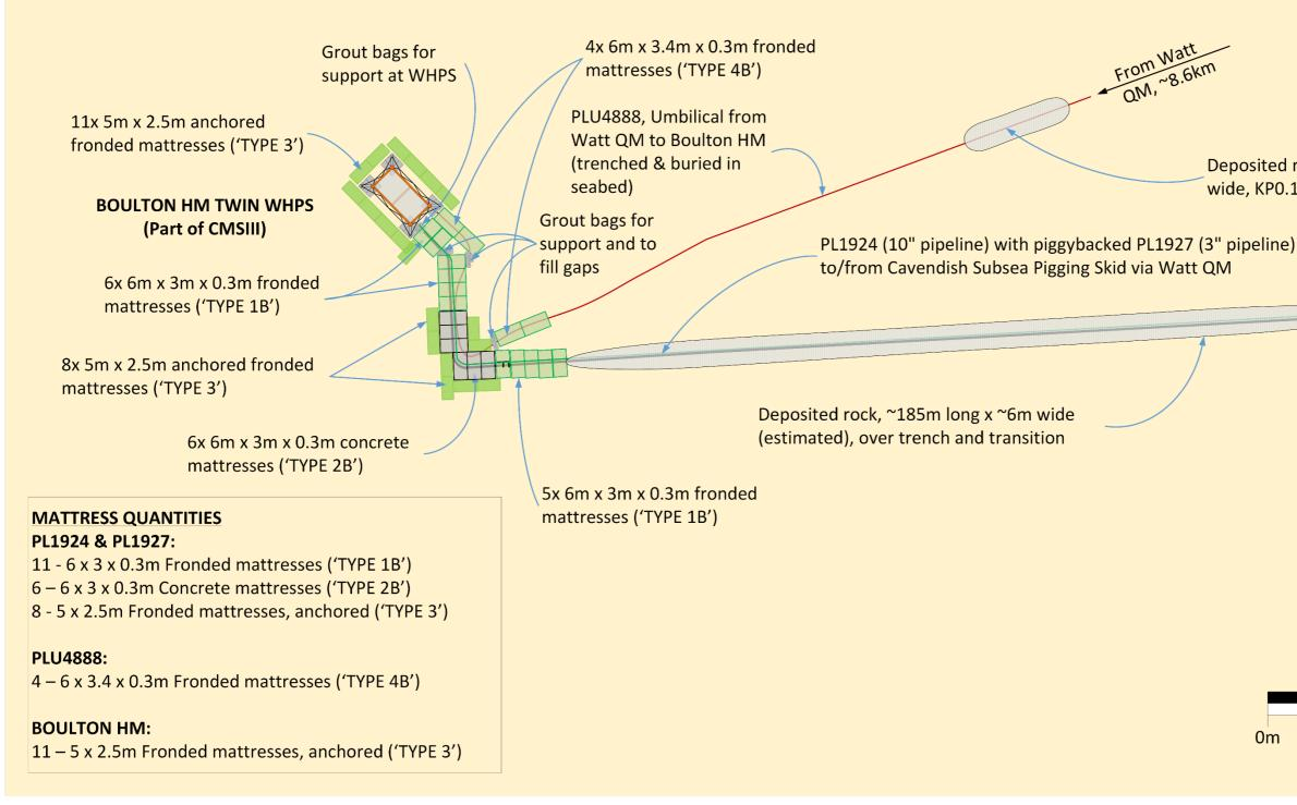
Figure A1.3.1: Schematic of pipelines near Boulton HM
