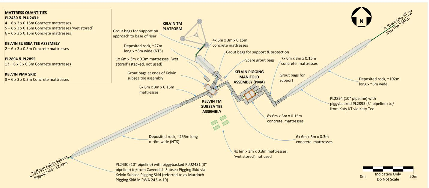
Figure A1.8.1: Schematic of pipelines near Kelvin TM
