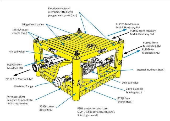
Figure 2.3.6: Perspective of the PSNL protection structure
