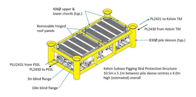
Figure 2.3.2: Perspective of the Kelvin/Murdoch Subsea Pigging Skid protection structure
