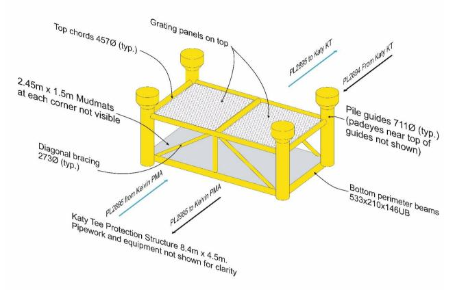
Figure 2.3.1: Perspective of the Katy Tee protection structure
