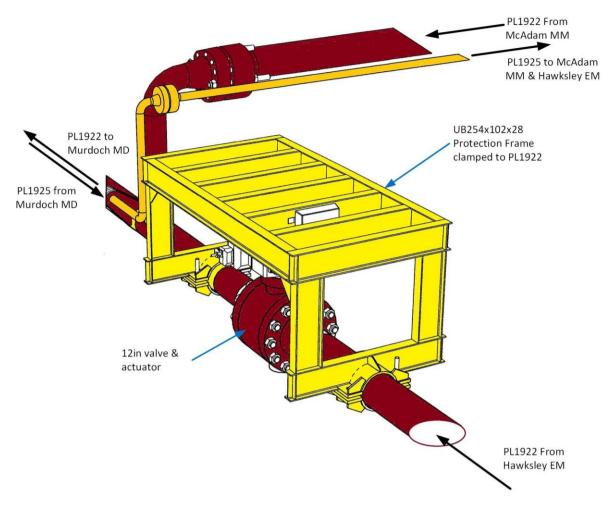
Figure 2.3.5: Perspective of the McAdam Tee protection structure
