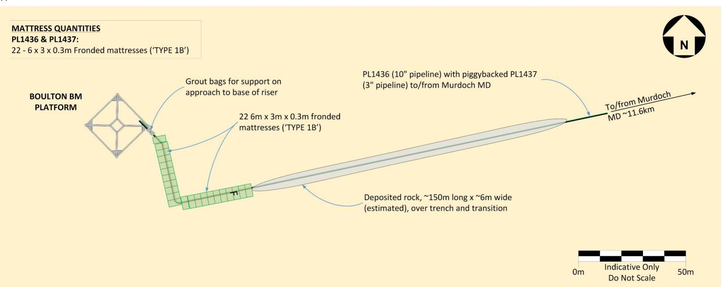
Figure A1.2.1: Schematic of pipelines near Boulton BM
