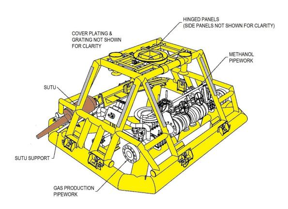
Figure 2.2.2: Perspective of Hawksley EM subsea installation
