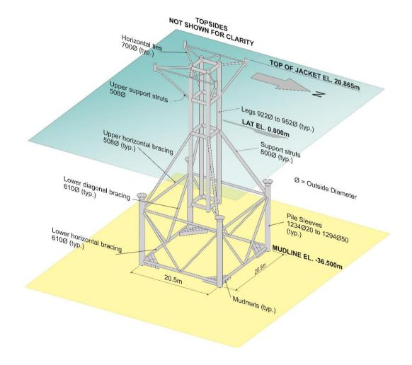
Figure 3.2.1: Boulton BM jacket 3D view
