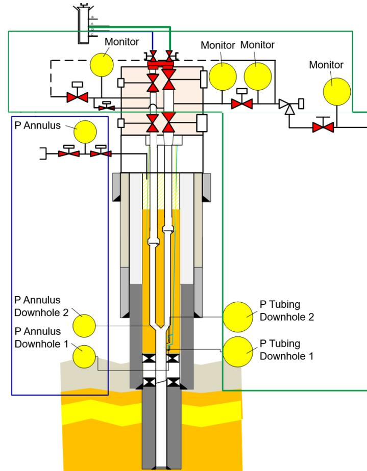
Figure 6-1: Well schematic
