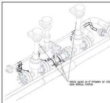
Figure 2-7 Tie-in Tee Protective Structure (Ref.6)
