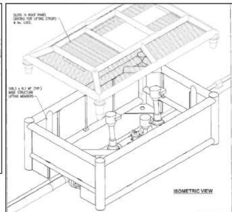
Fig A.14 Mid-line tee section diagram
