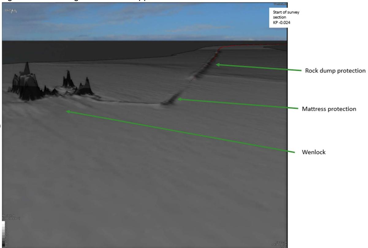
Fig A.9 Inde AC platform approach layout
