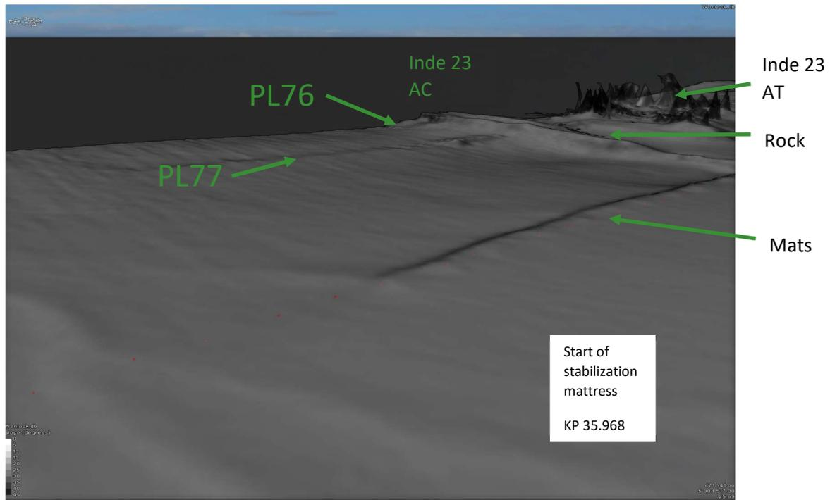
The 2020 pre decommissioning survey also confirmed the same status of mats and rock on the Inde AC approaches. The mattresses at both platform ends appear to have a very thin sediment covering with most concrete block rope linking loops visible.
