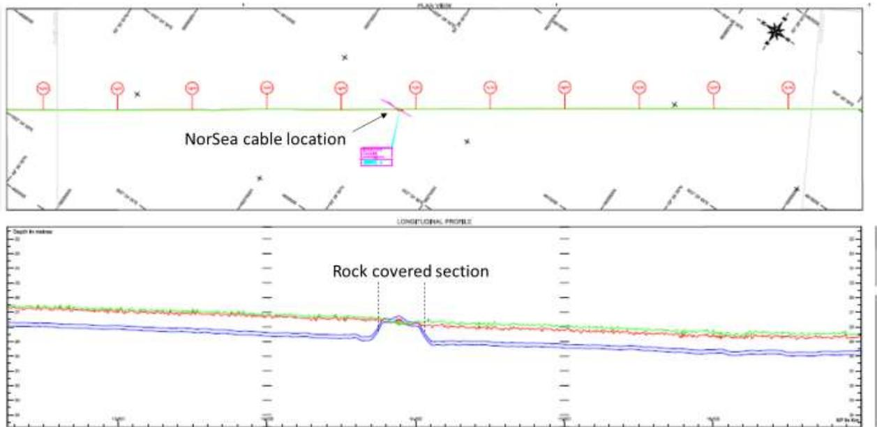
Fig A.5 2015 MBES image showing rock dump profile.
