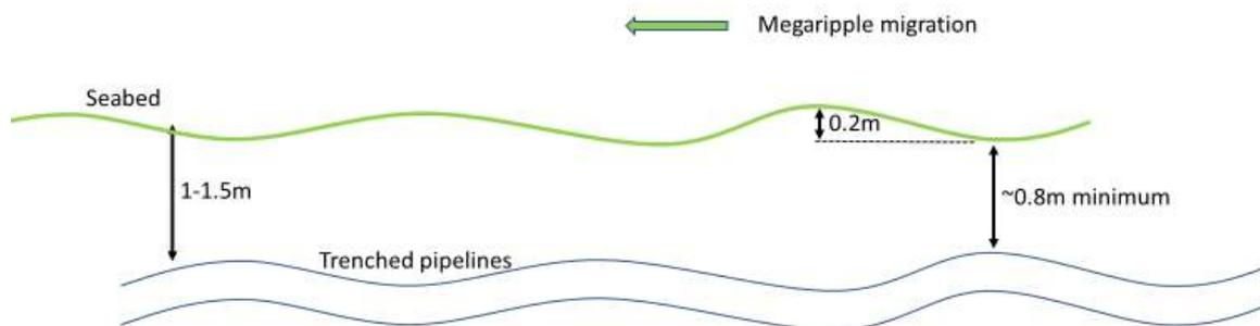
Even if mega ripples migrate the pipelines will still be >0.6m below the bottom of the megaripples.
