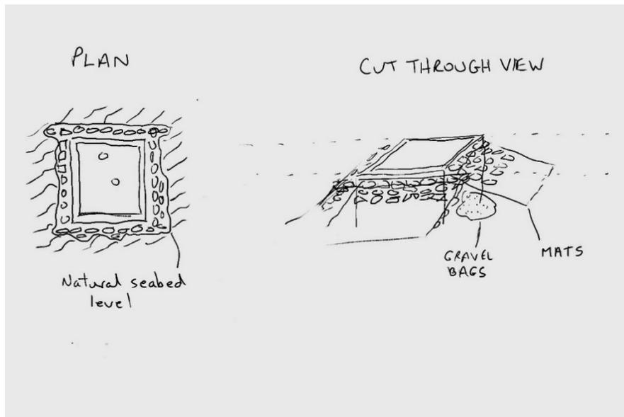
Seabed disturbance is reduced with this variance as the cover is not being lifted through any seabed material. The seabed surface area is also almost returned to its natural status with only the top of the structure tubulars remaining at the seabed surface. This combined with the reduced vessel time required resulted in a low overall environmental impact rating.
