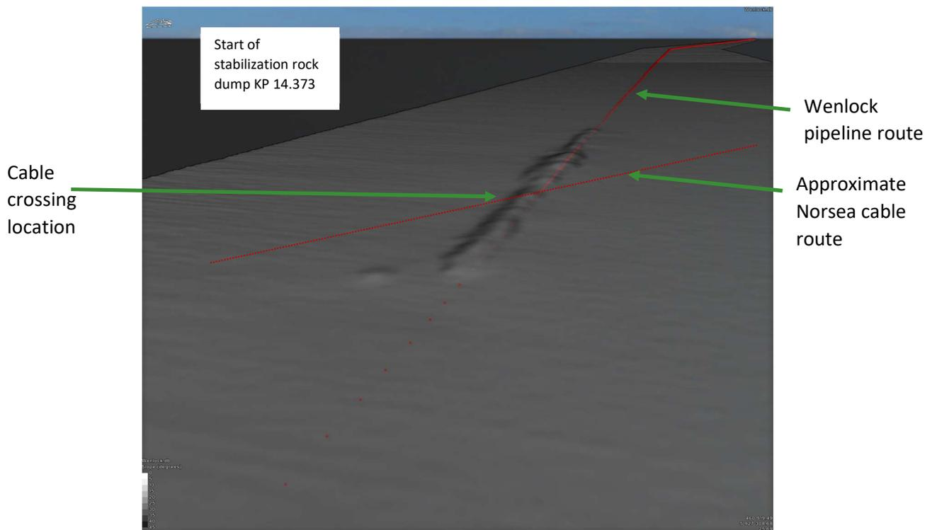
Fig A.6 below also shows the cable crossing location from the 2020 pre decommissioning survey with very little difference in the rock dump protection heaps. It appears that the rock is very stable in seabed currents and after fishing activity over the area.
