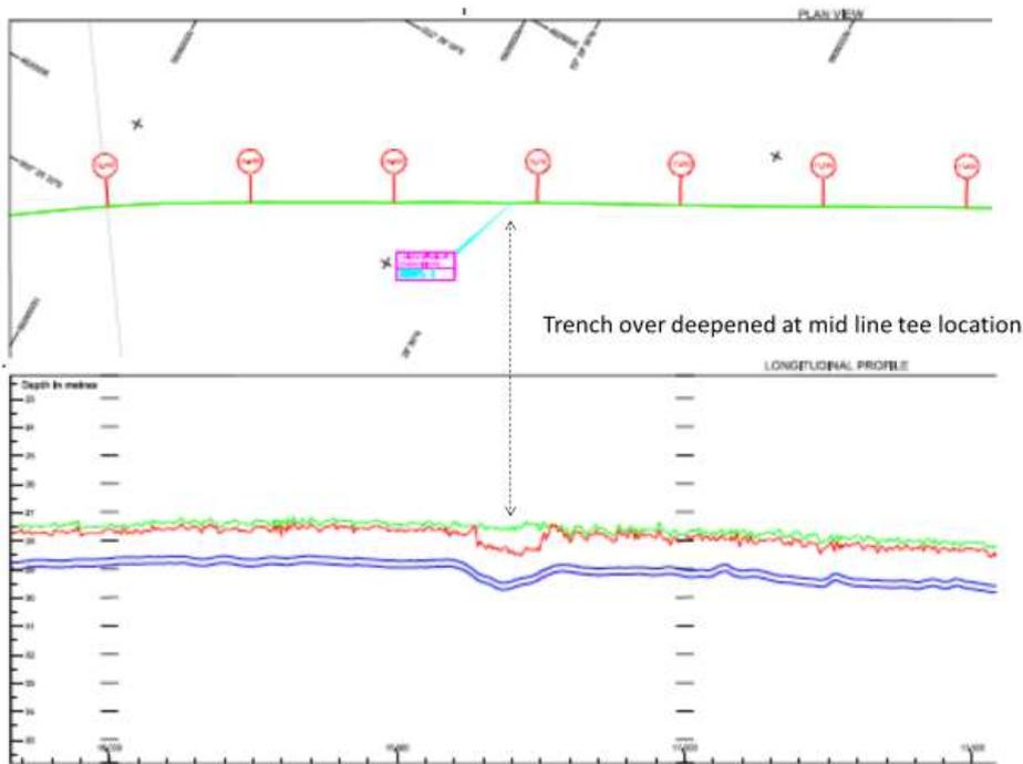
Fig A.13 Mid-line tee plan and sketches
