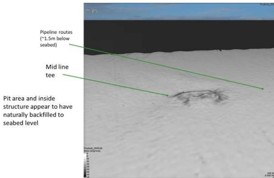
Video stills from the 2020 pre decommissioning survey of the internal structure shows the level of natural in fill to be at the same level as the surrounding natural seabed level.
