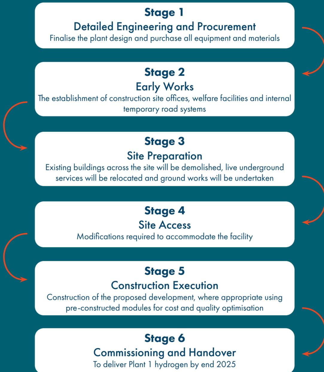
All stages of work will be required for Plant 1, whilst the construction of Plant 2 is expected to be largely a repeat of Stage 1, 5 and 6 as the enabling works for the plant will have been completed during the preparation for Plant 1. The Plant 1 schedule is shown in Figure 10.2, with an early indication of Plant 2 timing.
