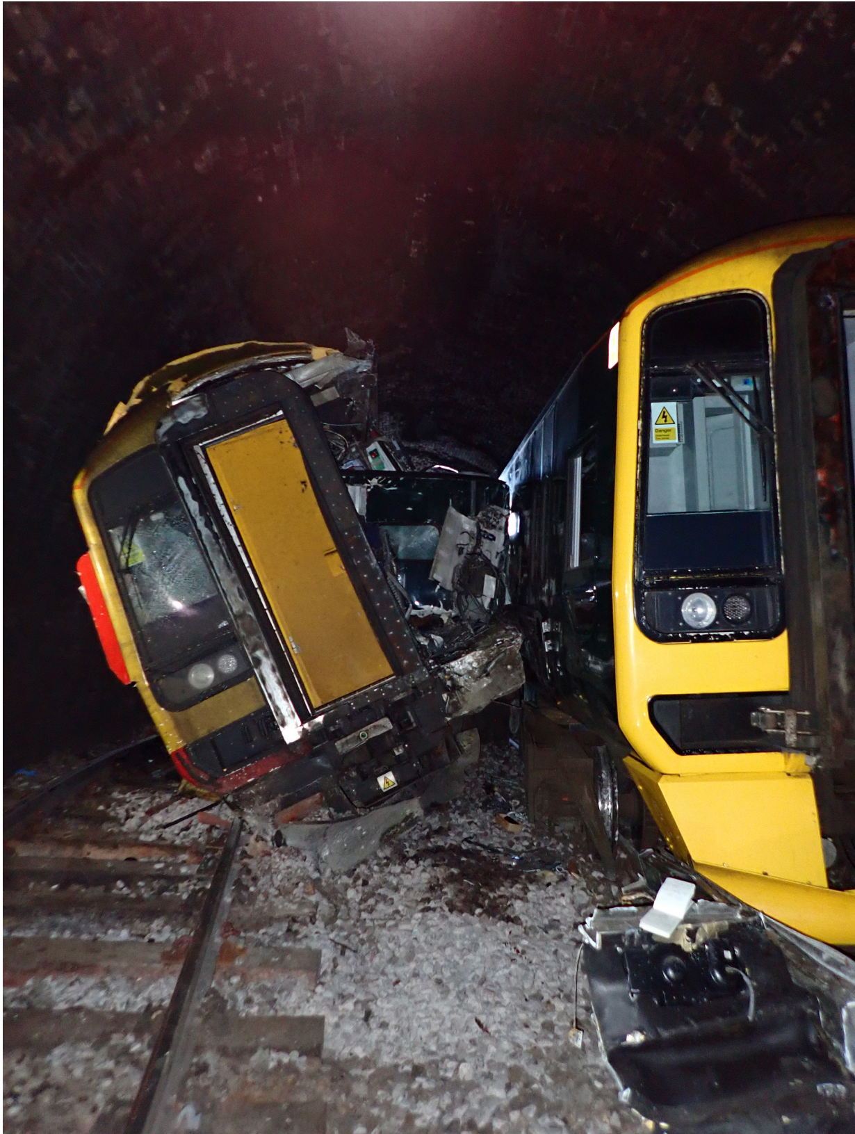
Figure 5: The scene inside the tunnel, showing the third coach of train 1F30 (right) and the leading coach of train 1L53 (left). Parts of the driving cab of train 1L53 have been cut away by the emergency services to release the trapped driver
