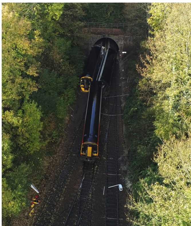
Figure 1: Aerial view of the trains involved once they came to a stand following the collision, showing the junction and tunnel mouth
