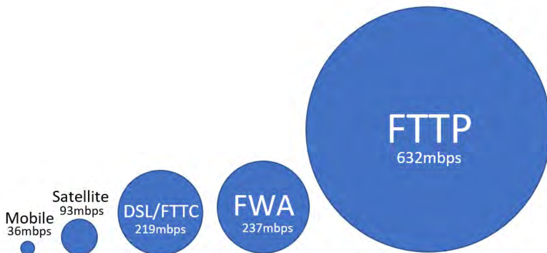
Figure 8.3: FTTP providers are able to deliver the highest average peak speed of any technology type, while satellites are able to deliver just below 100 Mbps.
