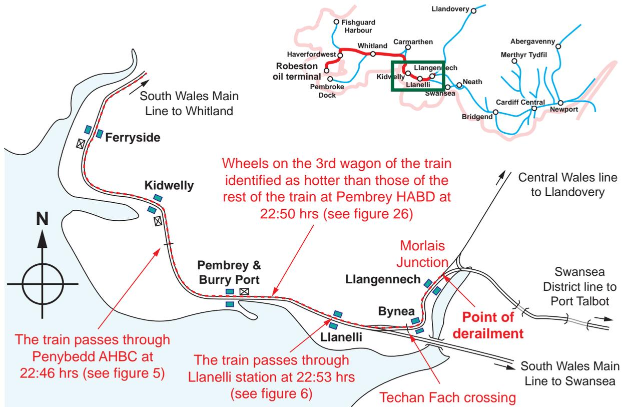
Figure 2: Map showing locations on the route from Robeston oil terminal to Morlais Junction
