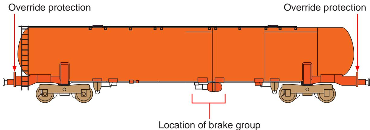
Figure 9: Diagram of a GF4-SS1 brake group on a GERS TEA type wagon
