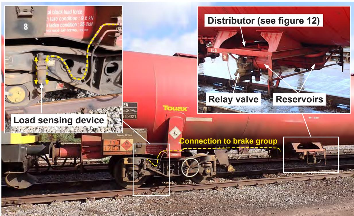
Figure 11: GF4-SS1 brake group on a TEA type wagon
