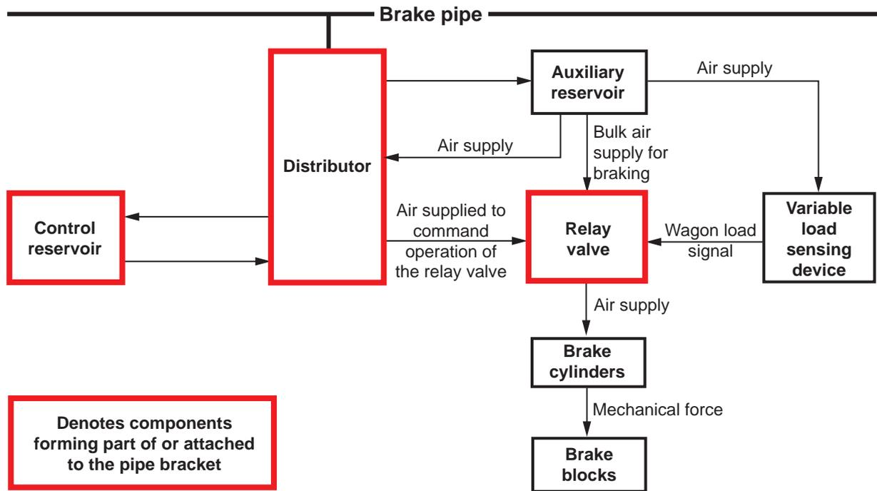
Figure 10: Schematic diagram of the wagon braking system showing the relationship between the various components including the distributor, control reservoir, auxiliary reservoir, relay valve, variable load sensing device, brake cylinders and brake blocks
