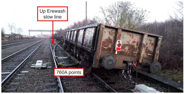
Figure 4: The derailed wagons (courtesy of DB Cargo)
