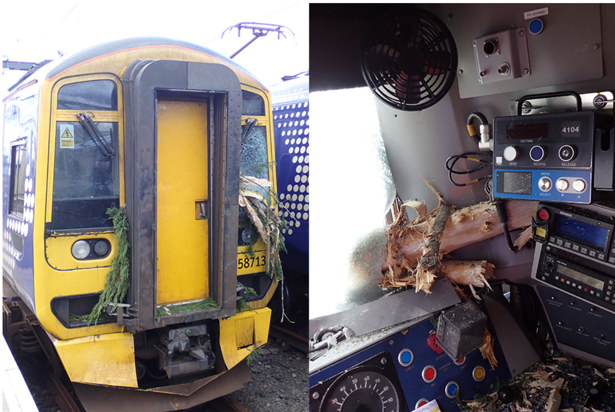
Damage to the driving cab of the train
