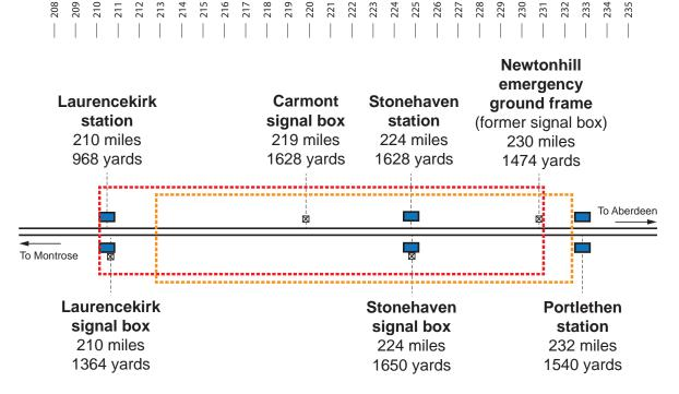
Figure 2: The BESR limits between Laurencekirk and Portlethen. The red box indicates the area defined by the locations on the form in the late notice case, the orange box the area defined by the mileages and intended by the asset managers (see paragraph 66).
