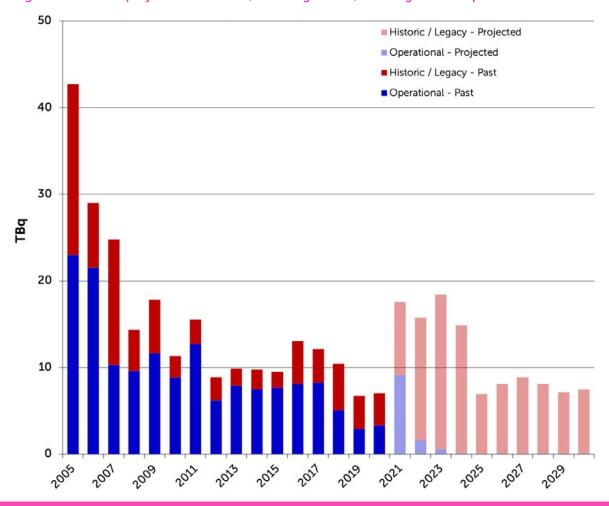
Figure 3. Past and projected tritium discharges from liquid effluents
