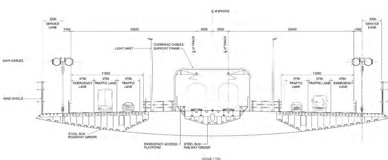
**Figure 14: Indicative bridge deck cross-section.**
