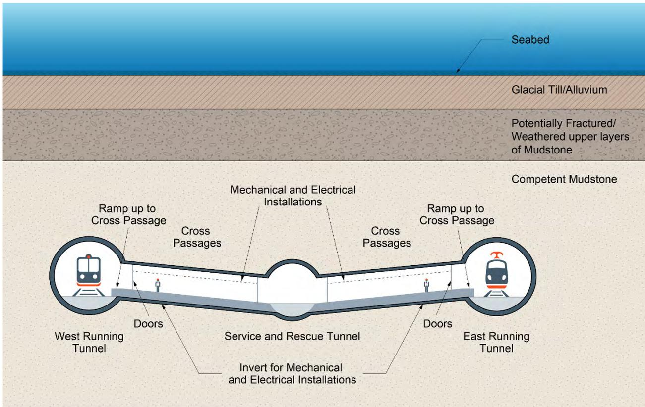
Figure 9: Indicative tunnel cross-section.
