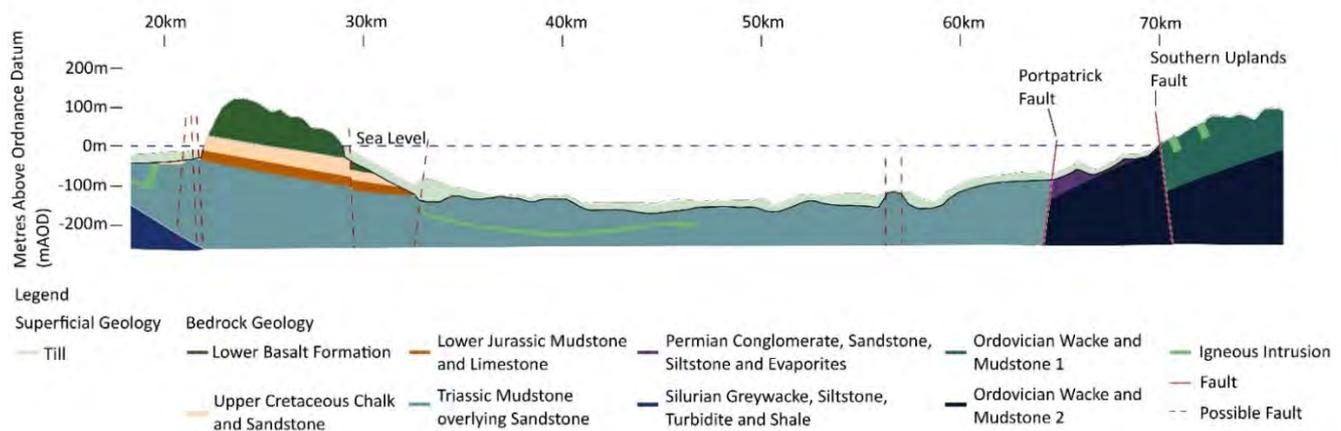
**Figure 7: Longitudinal section through indicative tunnel alignment.**
