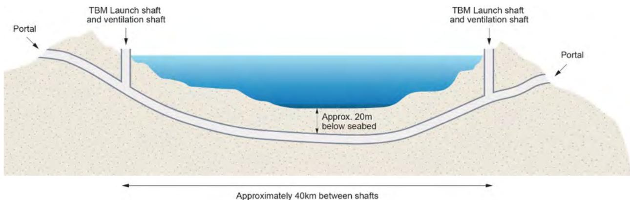
**Figure 8: Indicative tunnel vertical alignment.**
