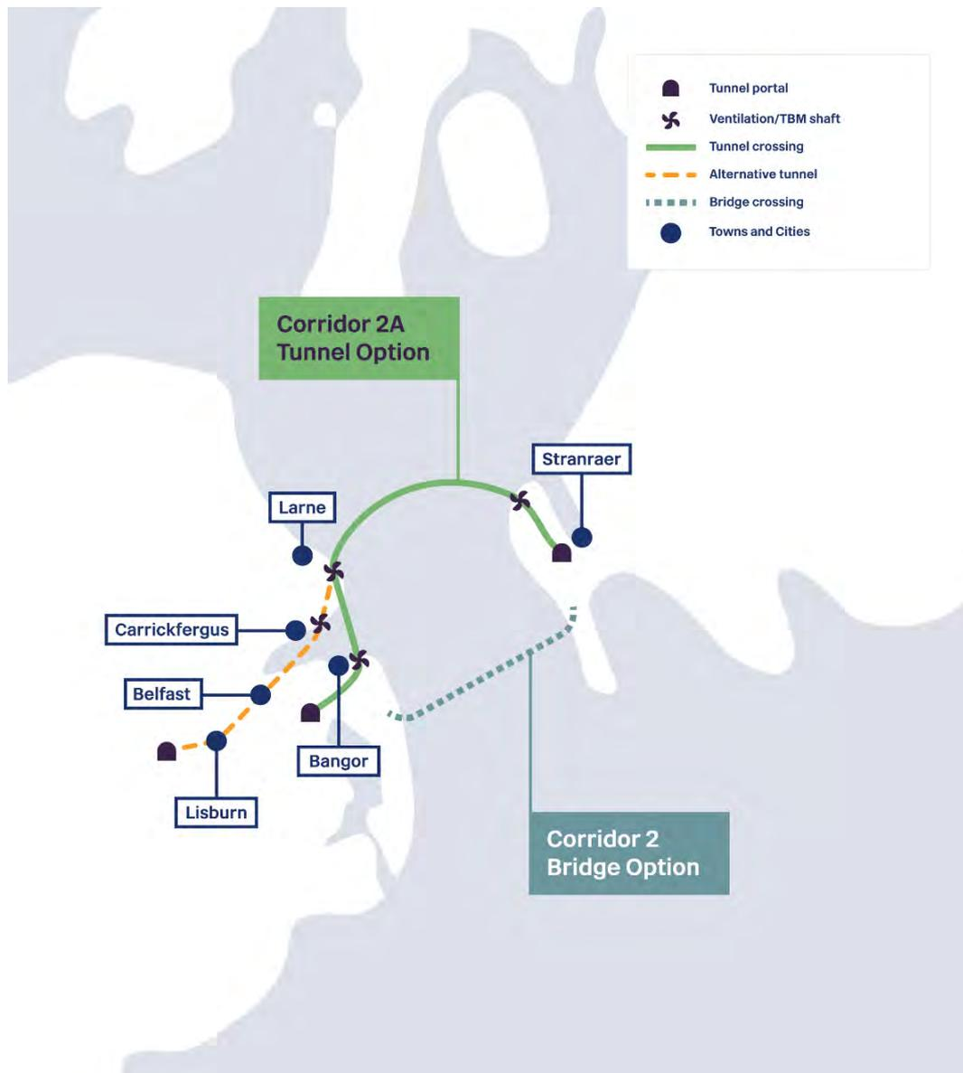
**Figure 5: Potential routes considered for tunnel and bridge crossings. Tunnel boring machine has been abbreviated to TBM in the key.**
