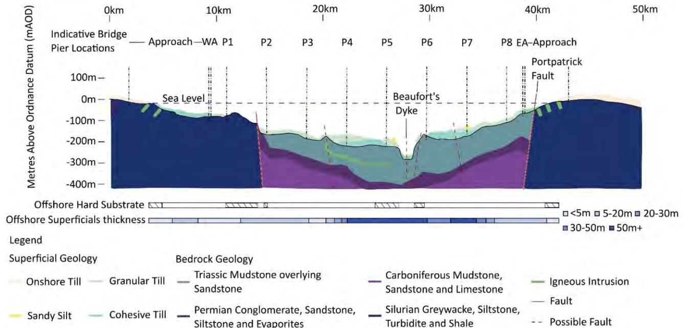
**Figure 12: Geological section through the North Channel approximately on the line of the bridge route.**
