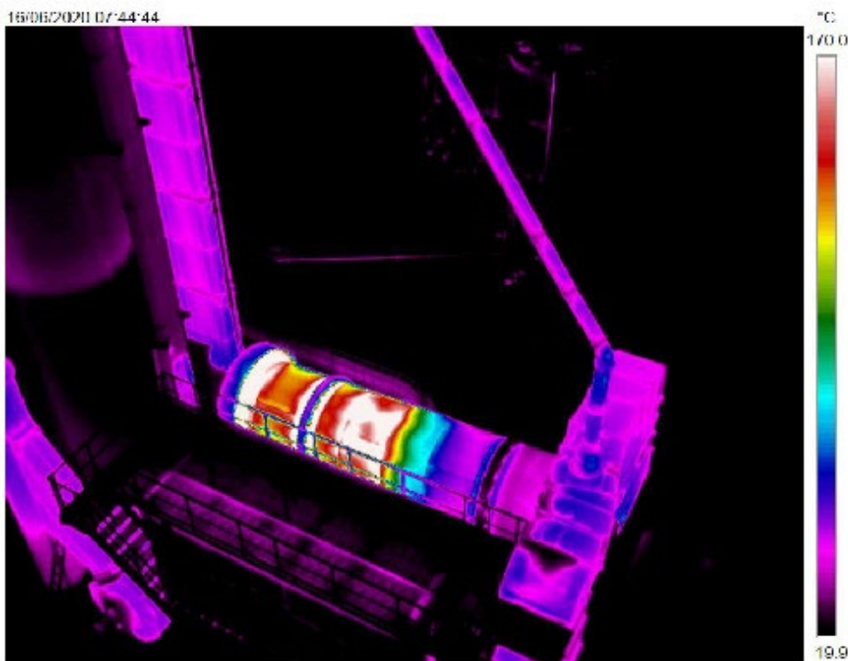
Thermal Image of Aggregate Heating Drum
