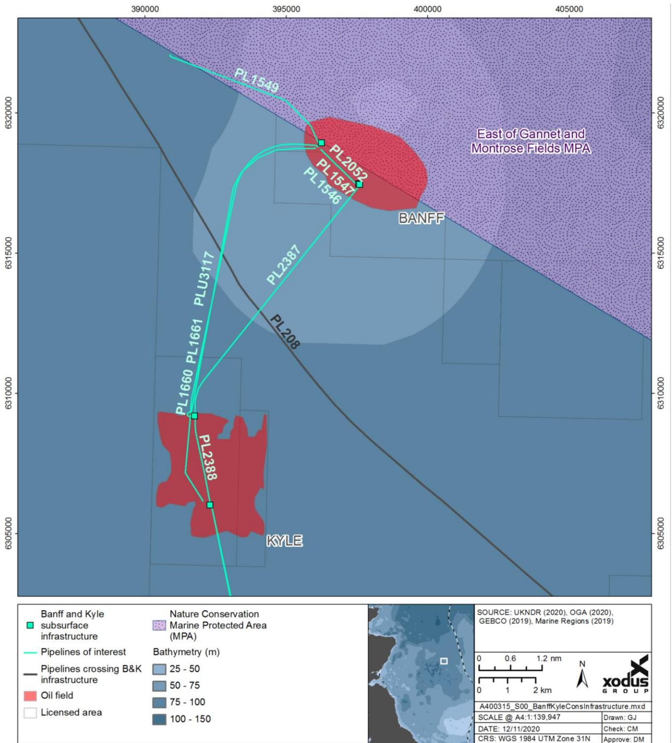
Figure 6-1 Pipelines within the Banff and Kyle Fields
