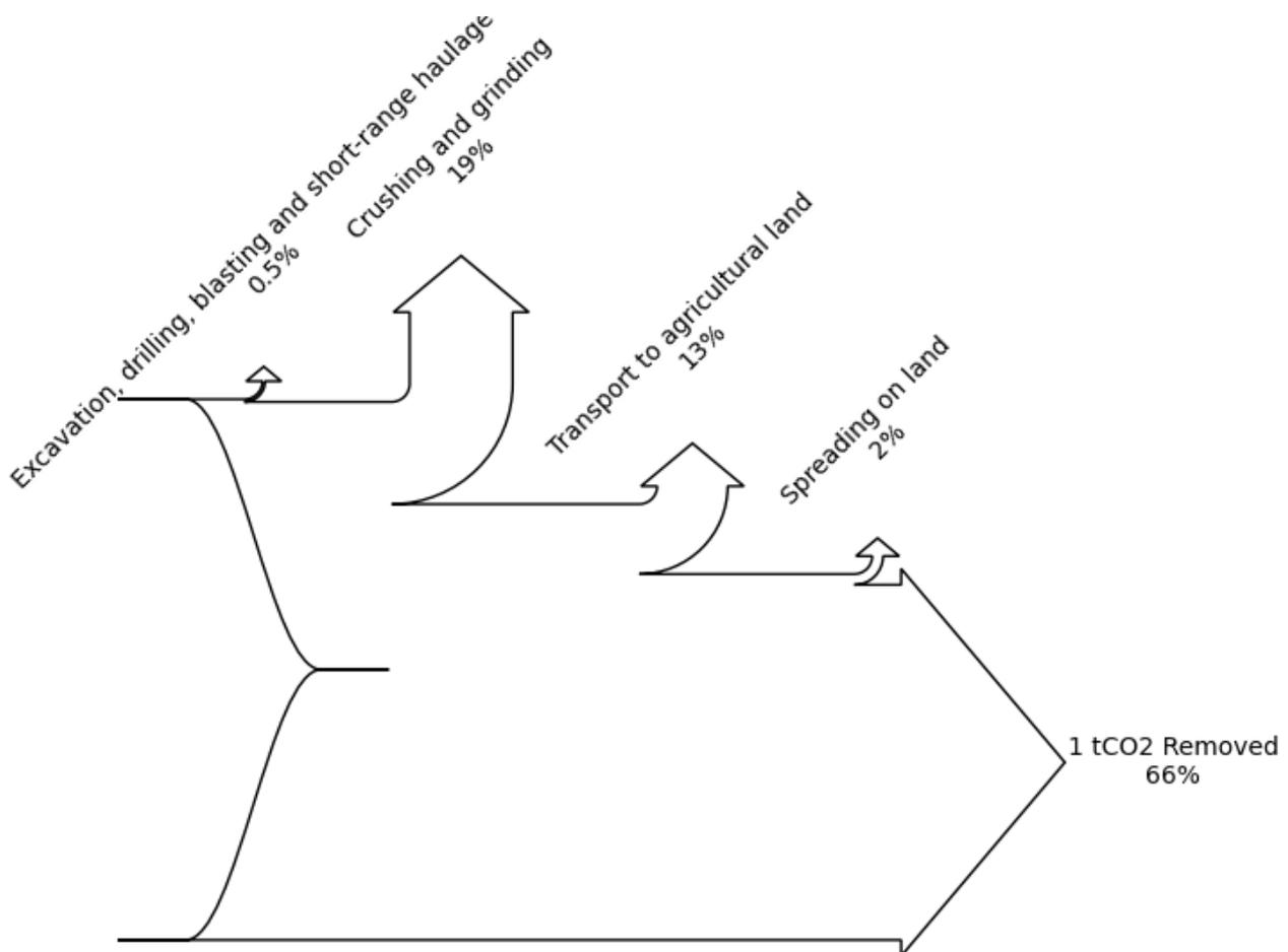
Figure 13: Illustrative carbon efficiency of passive enhanced weathering process. Here it is assumed that the mineral material is available in the UK. It can be observed that the primary sources of carbon leakage are the energy required for mineral size reduction, transport, and spreading on land.
