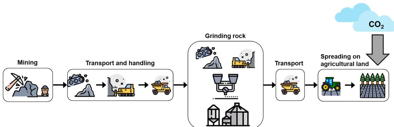
Figure 12: Illustrative flow diagram of an archetypal enhanced weathering (EW) value chain. Here, carbonate-able minerals, such as basalt or olivine, are mined, and then processed to produce a fine powder, which can be then transported and spread on available land. Subsequently, the carbonation of this material proceeds as a function of particle size, temperature, water, and time. CO<sub>2</sub> removed in this manner can be considered to be permanently removed.
