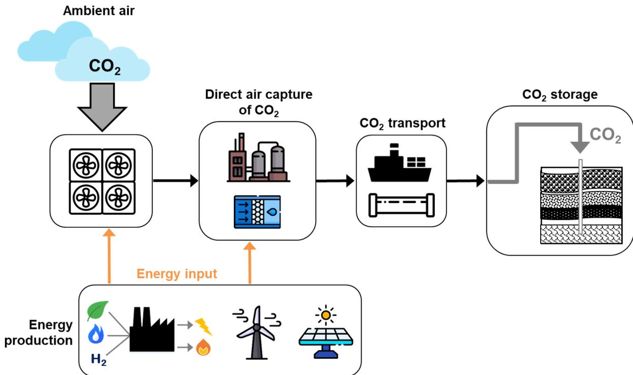
Figure 9: Illustrative flow diagram of an archetypal direct air carbon capture and storage (DACCS) value chain. Here the CO<sub>2</sub> is directly removed from ambient air, and subsequently transported to a geological storage facility.
