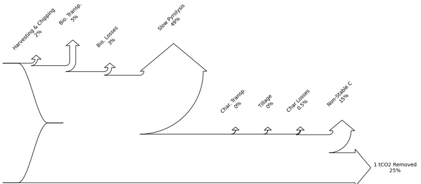
Figure 15: Illustrative carbon removal efficiency diagram for biochar application in the UK using forest residue from Scotland with char application in the midlands.
