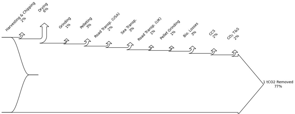
Figure 10: Illustrative carbon removal efficiency diagram for a UK BECCS project using biomass imported from the USA. This example assumes 98% CO<sub>2</sub> capture. At 90% capture rate, the carbon removal efficiency is reduced to approximately 70%.
