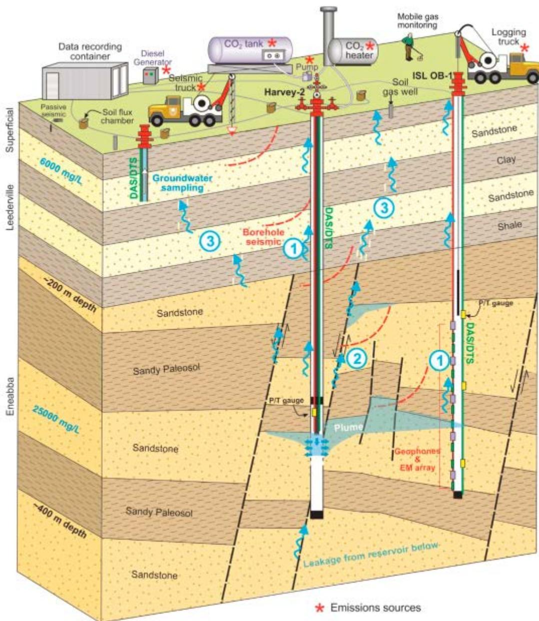
**Figure 64: Potential leakage pathways to the ground surface 1) leakage along the well due to inadequate cementing 2) leakage along faults and 3) leakage along zones of increased permeability (Mayers, et al., 2020)**
