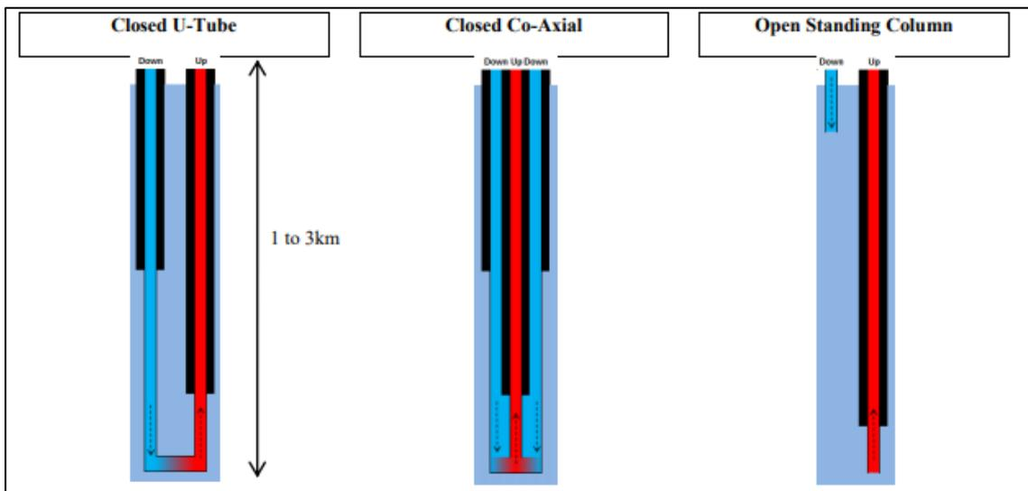
**Figure 38: Configurations considered for a DGSW configuration (Law and others, 2016).**
