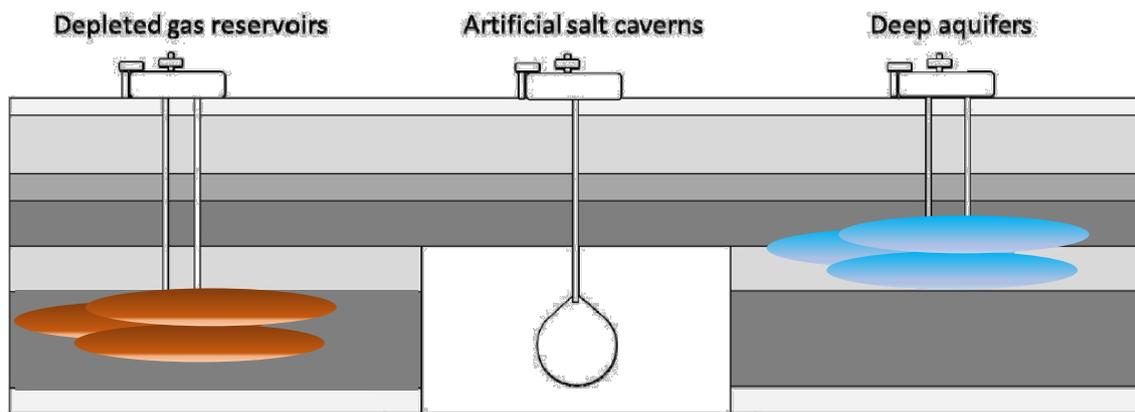
**Figure 16: Schematic depiction of the 3 major types of UHS. Diagram not to scale. Brown & light blue shading indicates porous rock, white box indicates salt deposits (Dopffel and others, 2021)**
