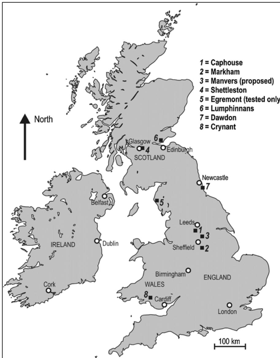
**Figure 30: Overview map of Britain and Ireland, showing mine water heat pump schemes. The Egremont setup is based on an ironstone (haematite) mine, while the rest are coal mines (Banks and others, 2019)**
