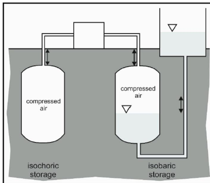
**Figure 10: Schematic of operational isochoric (constant volume) and isobaric (constant pressure) pressure modes in underground storage of CAES (Evans & Carpenter, 2019)**
