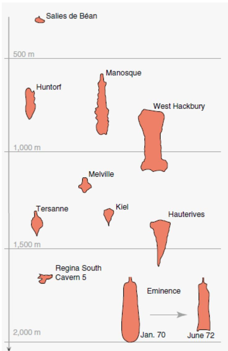
Figure 13: Depth profiles of various salt caverns, all are in salt domes except Regina South and Salies de Bean, which are in bedded salt (Warren, 2016)
