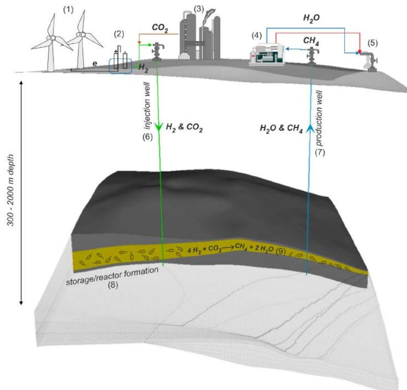
**Figure 17: The concept of a doublet system for underground bio-methanation (Strobel and others, 2020)**
