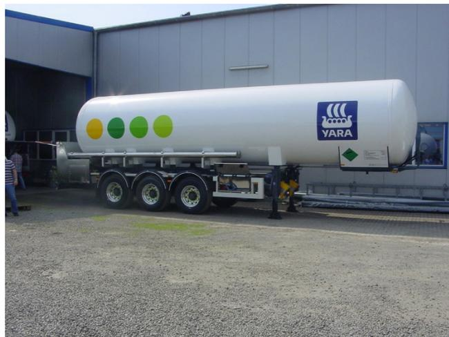
**Figure 20: A road tanker for CO<sub>2</sub> transport used in the fertiliser manufacturing industry in Europe (Van Hool Road Tankers, 2021)**
