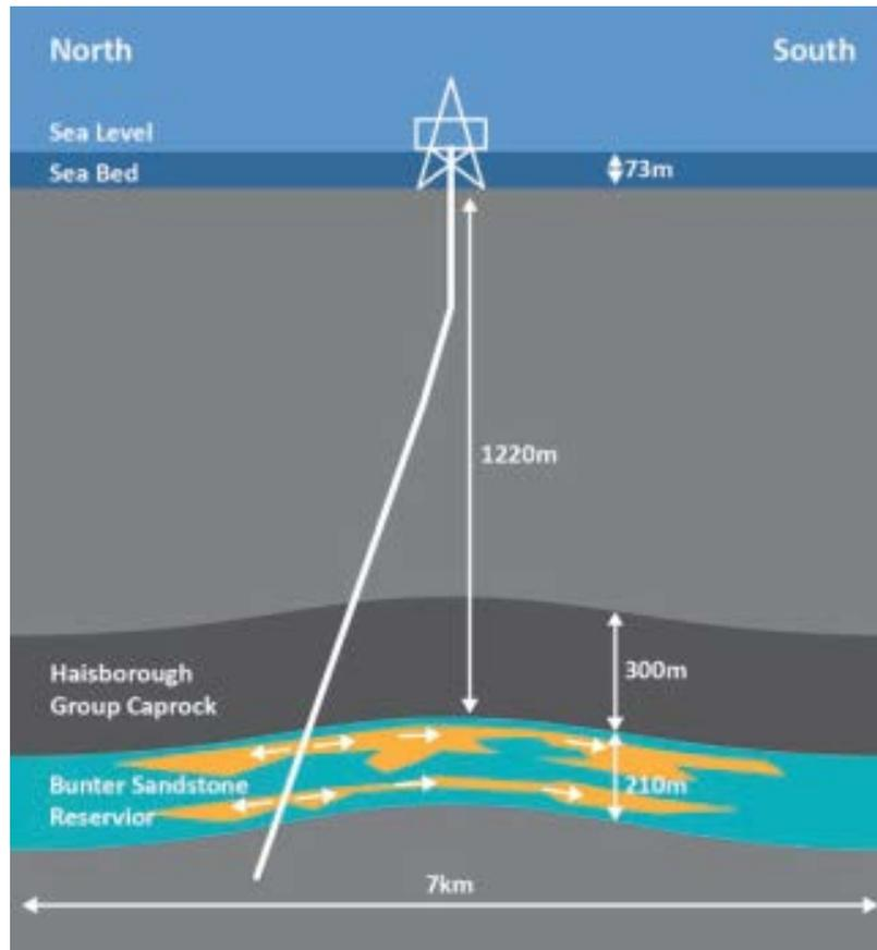
**Figure 27: Bunter Closure 36 saline aquifer dome in the Southern North Sea. Yellow indicates the potential storage formation. Blue indicates saline fluids. Rig not to scale (Pale Blue Dot, 2016)**
