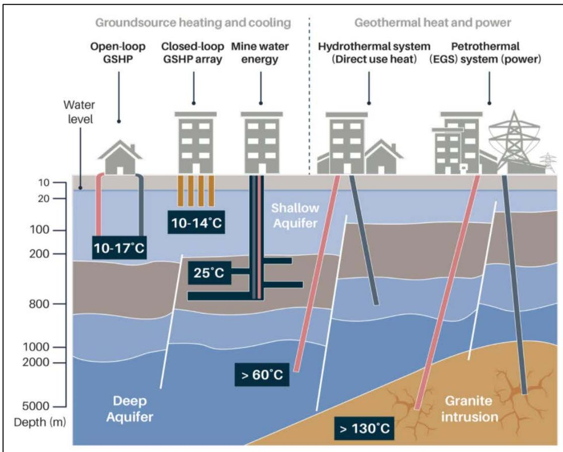
**Figure 29: The various options regarding geothermal energy extraction (Abesser et al., 2020)**
