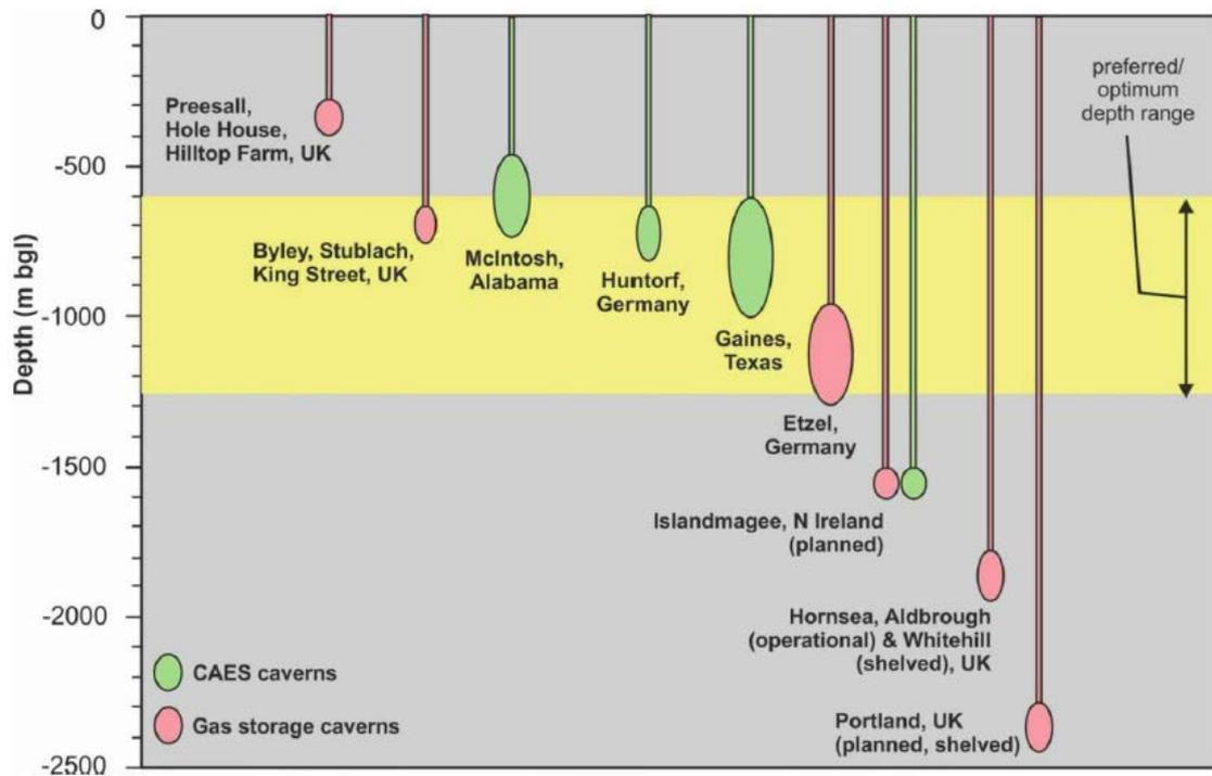
**Figure 6: Selected example to illustrate the depths of operational and proposed global gas storage caverns and operational and proposed global CAES caverns (Parkes and others, 2018)**
