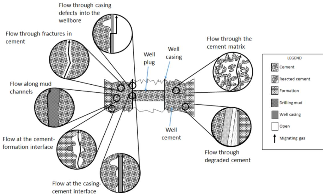
**Figure 23: Schematic of potential well integrity issues for CO<sub>2</sub> injection wells (Sminchak, 2018)**
