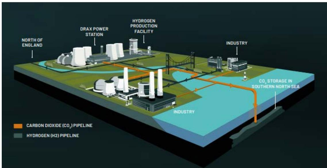
**Figure 50: Schematic illustration of the Zero Carbon Humber project, including hydrogen reformation (Zero Carbon Humber, 2020)**
