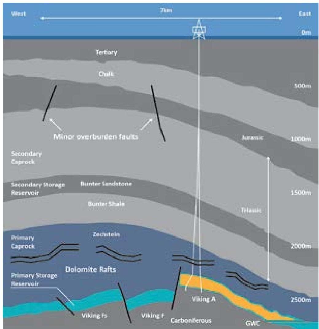
**Figure 26: Viking depleted gas field in the Southern North Sea. Yellow indicates the potential storage formation. Rig not to scale (Pale Blue Dot, 2016)**
