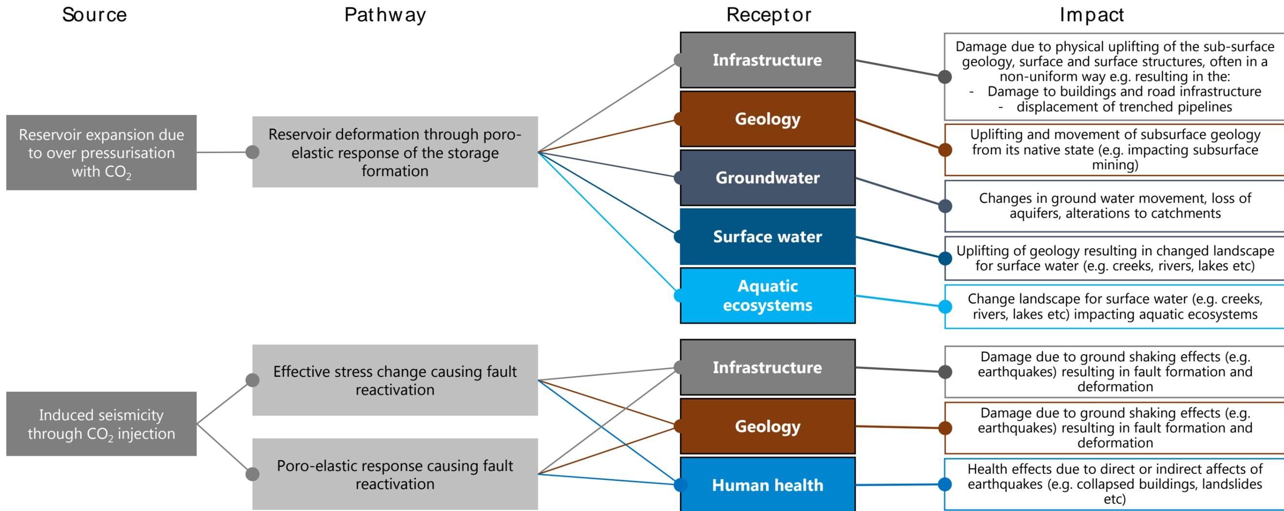
Figure 69: SPR diagram for physical impacts from CO<sub>2</sub> injection
