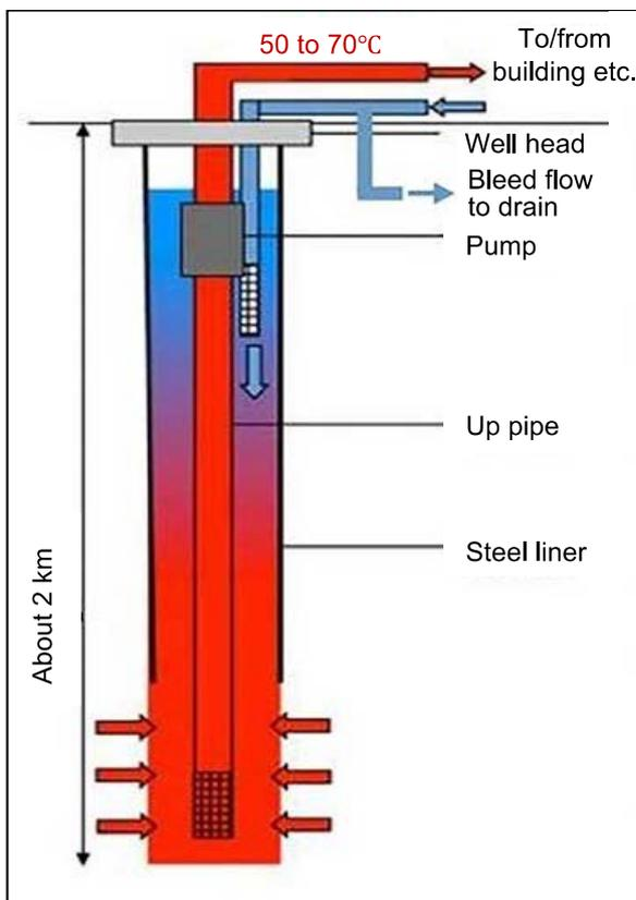
**Figure 37: Schematics of the DGSW technology tested in Rosemanowes, Cornwall (Collins & Law, 2017)**
