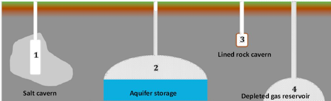
**Figure 11: 4 types of CAES underground storage options (adapted from (King and others, 2021)). Mined voids are not shown and grey shading in 2 and 4 indicates porous rock. Diagram not to scale.**
