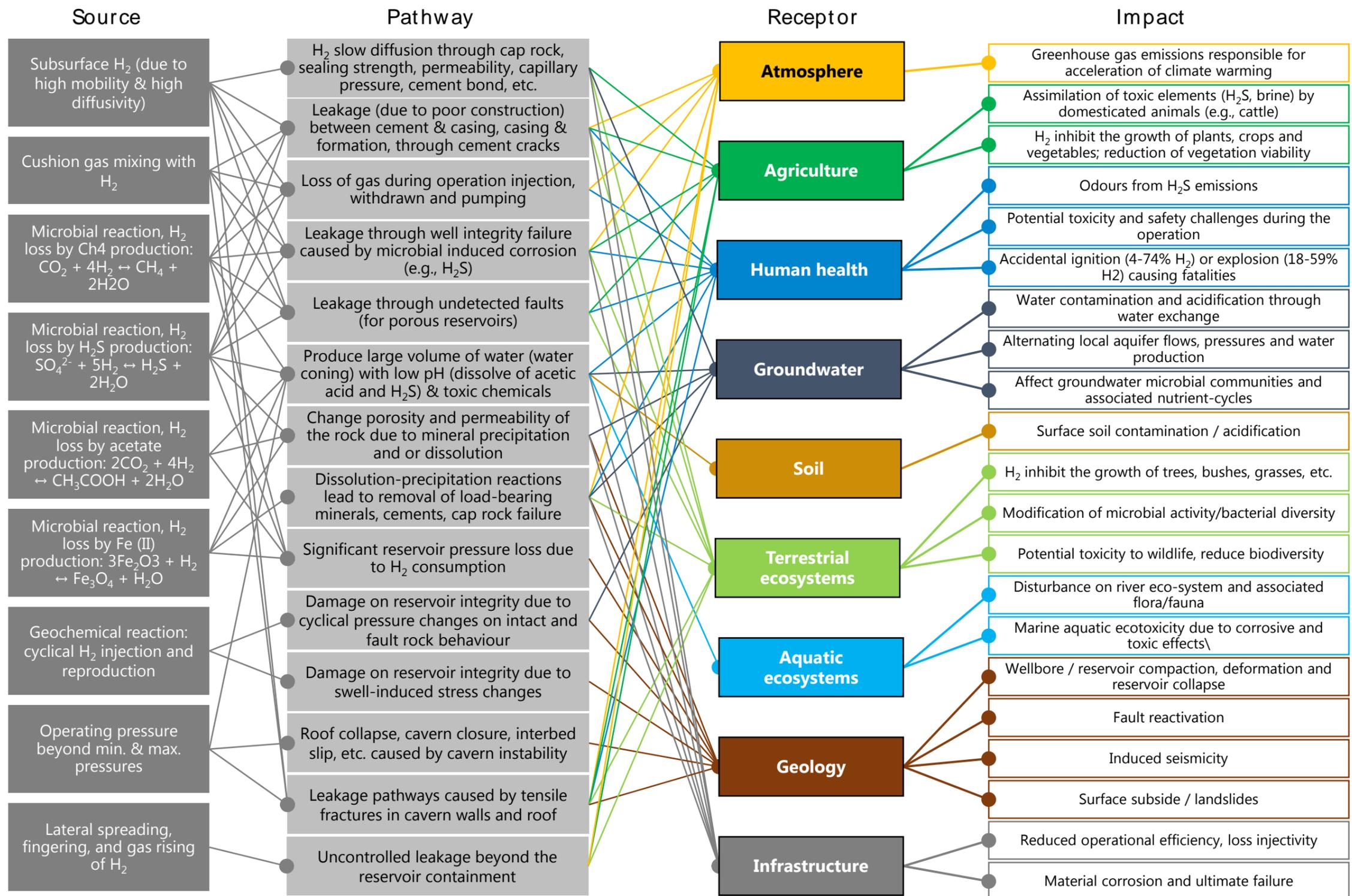
Figure 62: SPR diagram for UHS operation (excluding site preparation)
