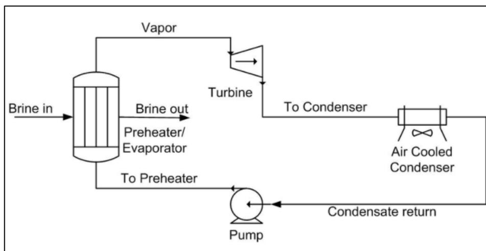
**Figure 5: Basic schematic diagram of a binary plant (Ashwood & Bharathan, 2011).**
