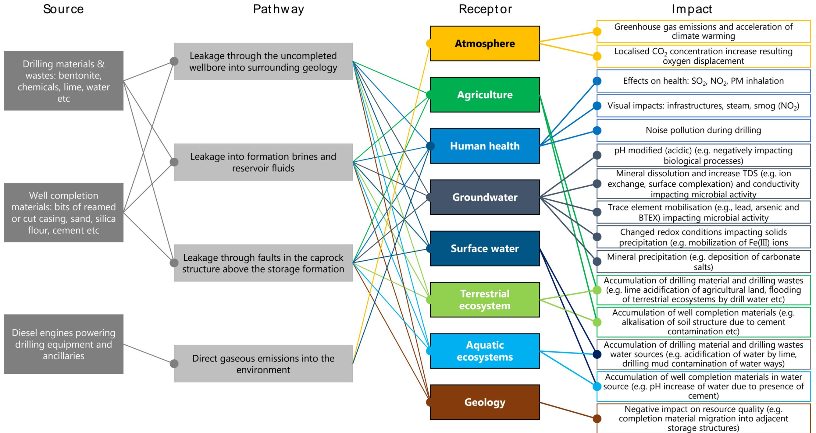
Figure 67: SPR diagram for CO<sub>2</sub> injection well drilling and preparation
