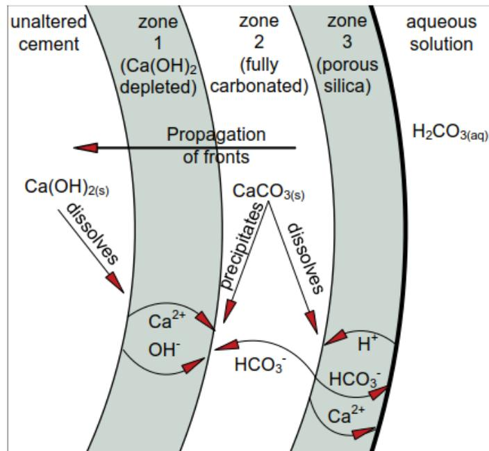
**Figure 25: Illustration of cement degradation due to carbonic acid attack (Medimuric, 2010)**
