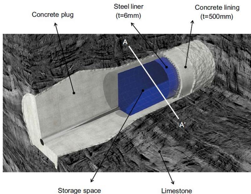
**Figure 15: A CAES pilot test cavern located in limestone at a depth of about 100m (Kim and others, 2016).**
