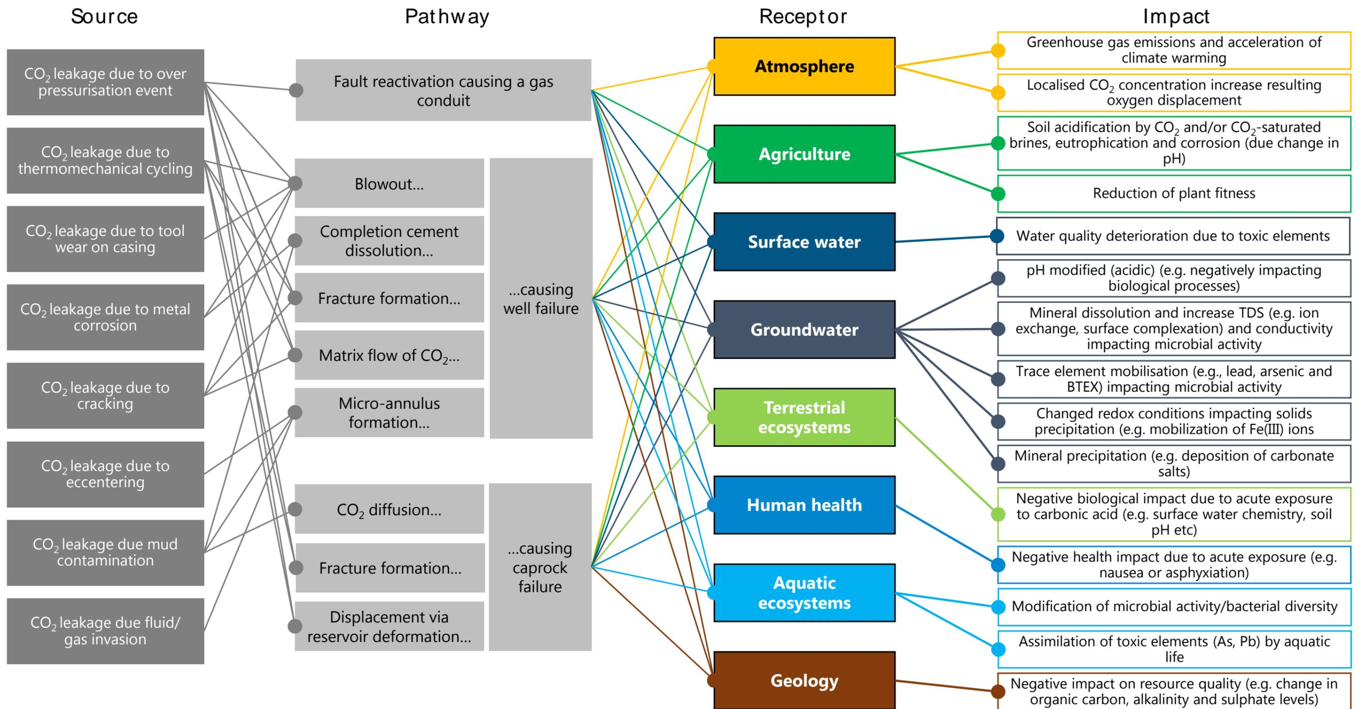
Figure 68: SPR diagram for CO<sub>2</sub> leakage from storage formation
