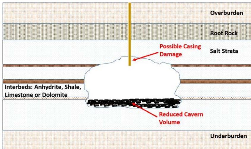
**Figure 56: Consequences of interbed slip: casing damage and reduction in volume (Duhan, 2018)**
