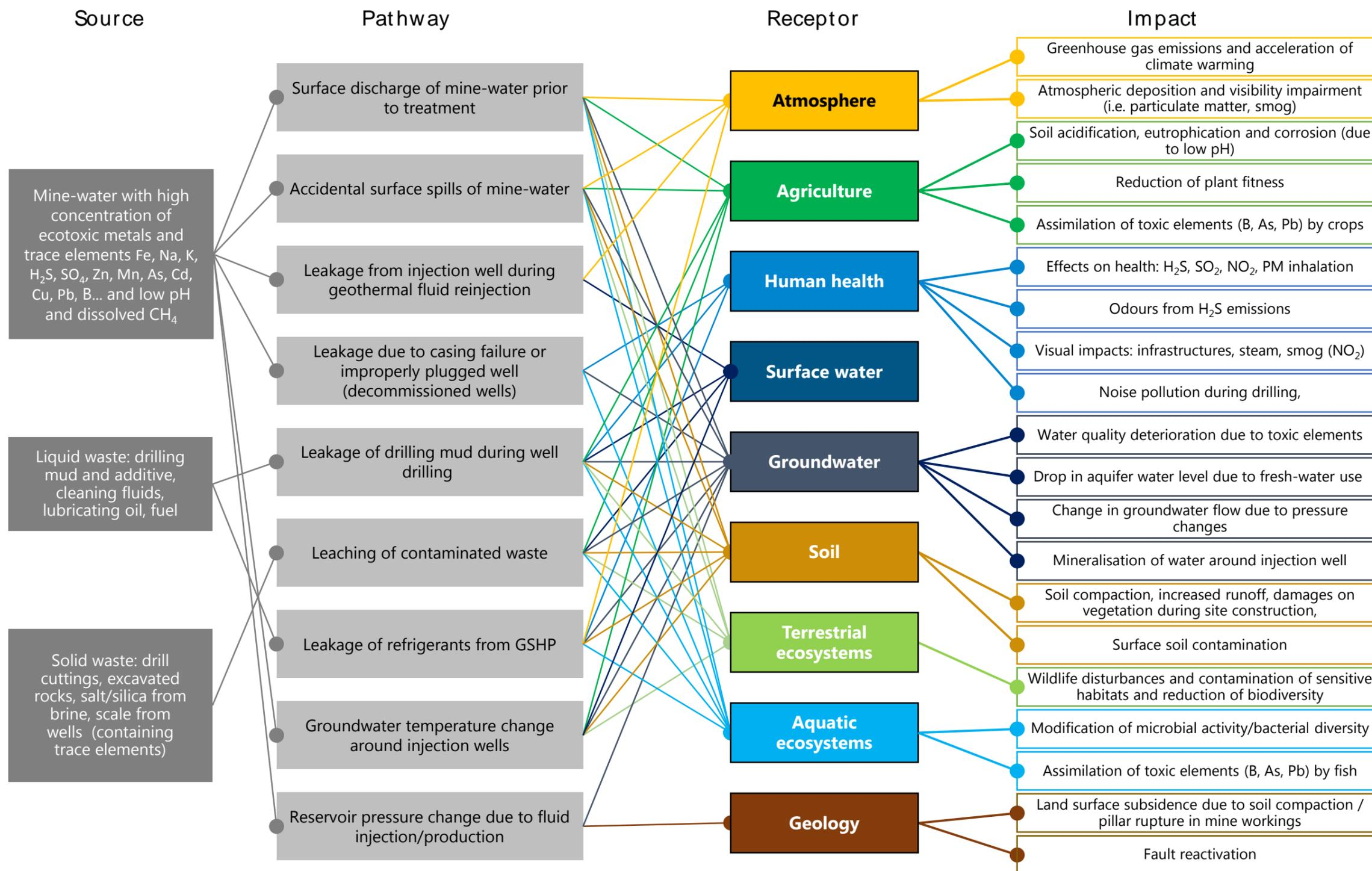
Figure 53: SPR diagram for mine water geothermal heating and cooling
