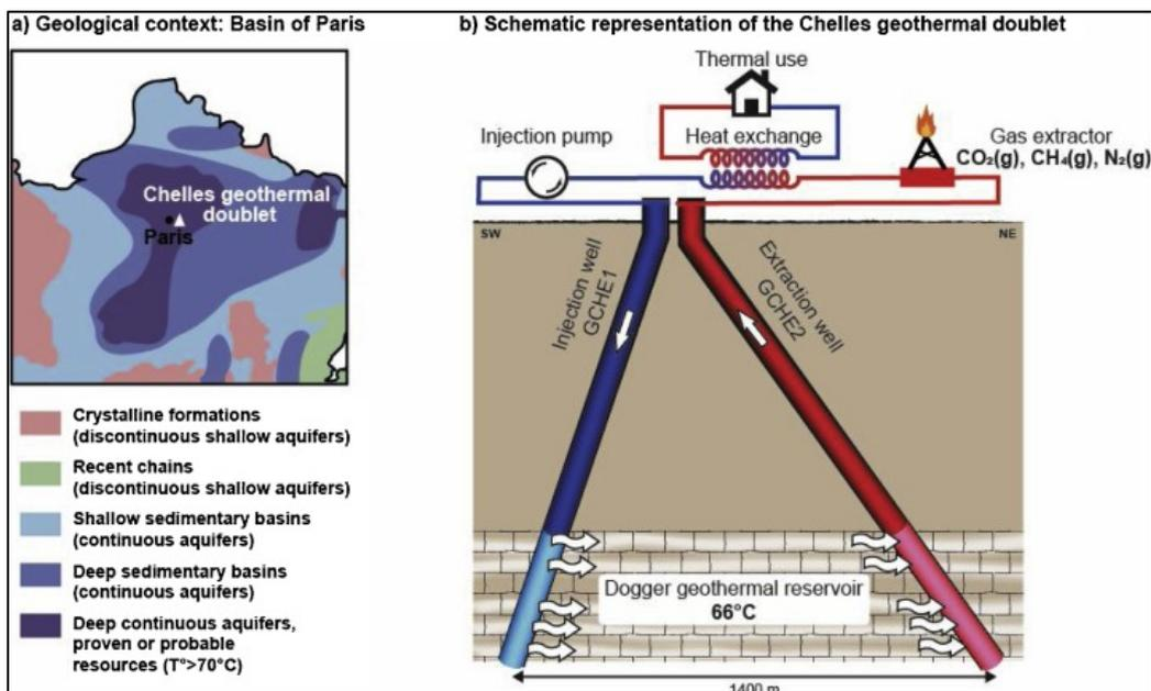
**Figure 6: Schematic of the setup in the Dogger carbonate aquifer in the Paris Basin (Marty and others, 2020)**
