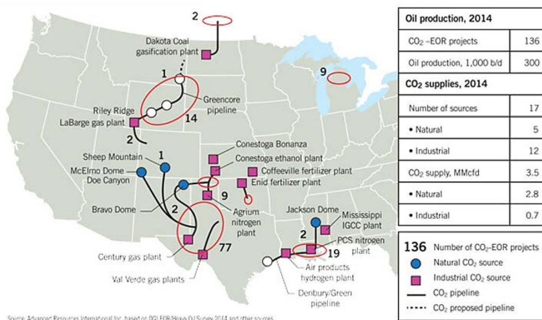
**Figure 44: United States (Weyburn storage project in Canada is connected with a North Dakota CO<sub>2</sub> source) CO<sub>2</sub>EOR infrastructure and operational projects (Oil & Gas Journal, 2014)**
