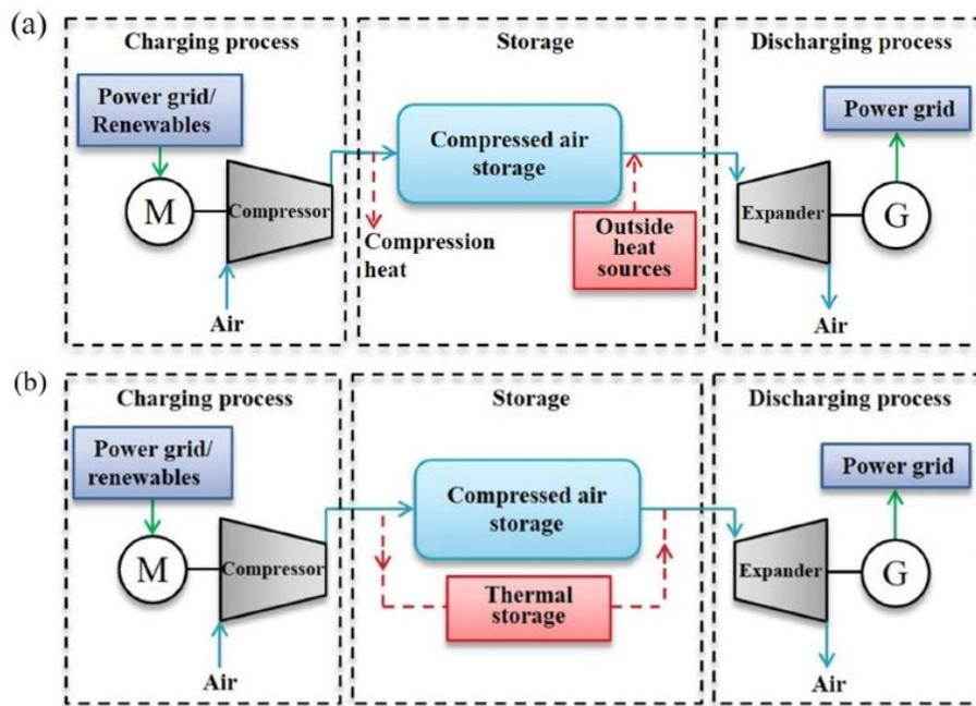
**Figure 9: Comparison between (a) D-CAES; and (b) and A-CAES (M – Motor, G – Generator) (Tong and others, 2021)**
