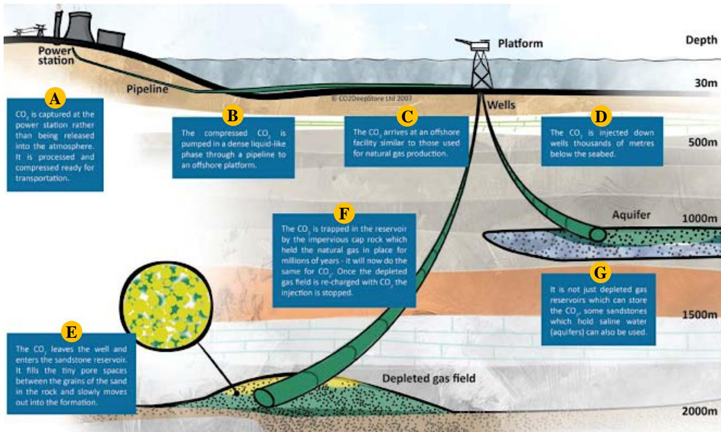
Figure 19: Schematic of the CCS process, including storage within a saline aquifer and depleted natural gas field (Pale Blue Dot, 2016)
