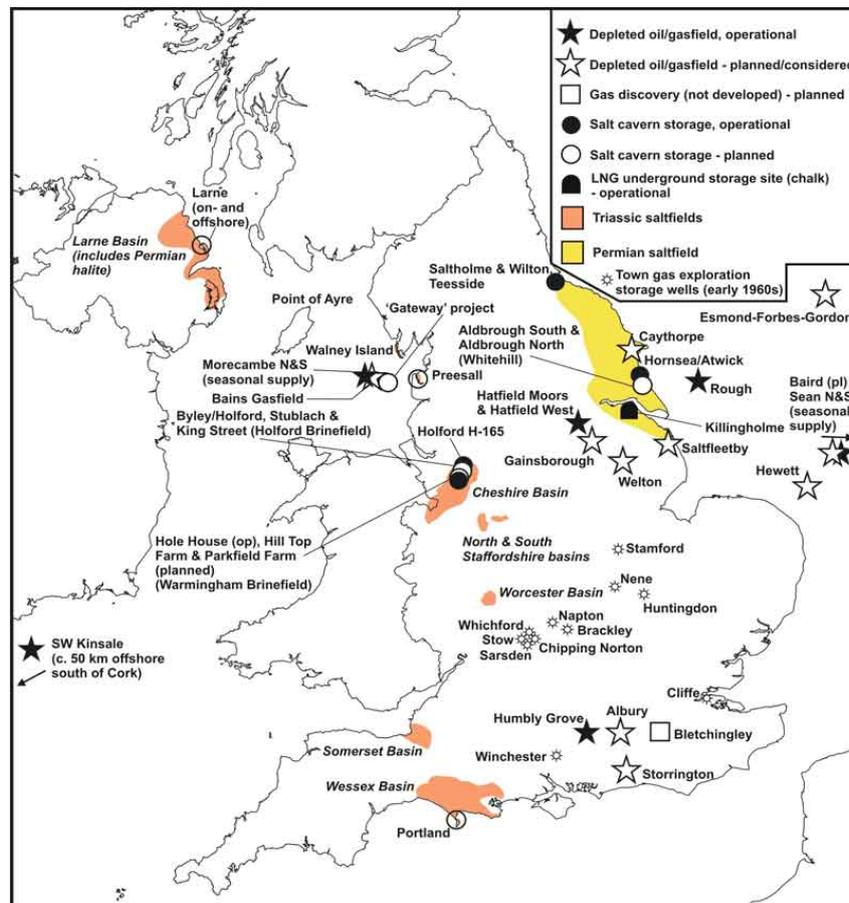
**Figure 41: Distribution of the main halite-bearing basins in England (and Northern Ireland) and the location of operational and proposed underground gas storage sites, including depleting oil and gas fields and mined chalk facilities (Evans & Holloway, 2009)**
