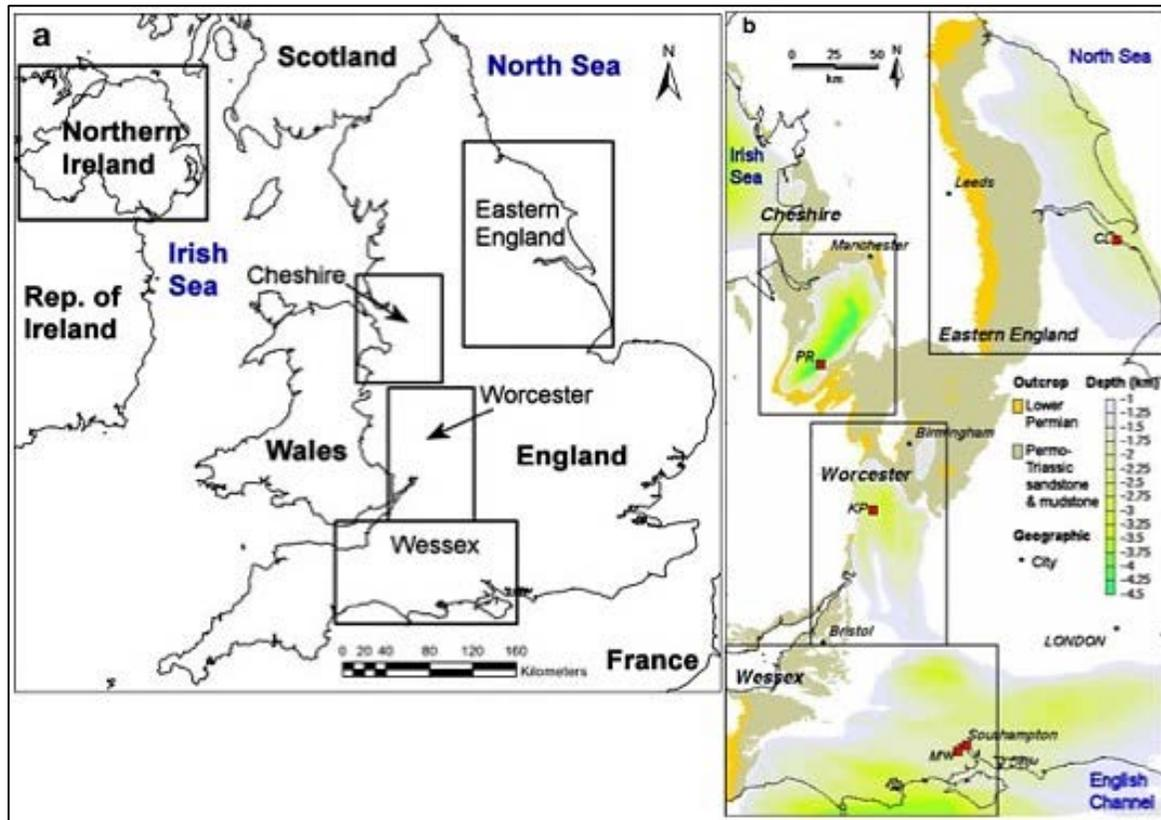
Figure 34: Main Mesozoic basins within the UK- (a) general location map of the eastern England, Wessex, Worcester and Cheshire Basins in England (and partly Wales) shown with depth to base of the Permo-Triassic sandstones. Red squares are deep boreholes referred to in the text: CL Cleethorpes; KP Kempsey; LA Larne No. 2; MW Marchwood; PR Prees; and Southampton) (Busby, 2014)
