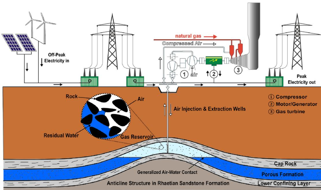
**Figure 8: A schematic sketch of a hypothetical conventional CAES facility using a porous formation as the storage reservoir. Diagram not to scale (Bo Wang, 2019).**
