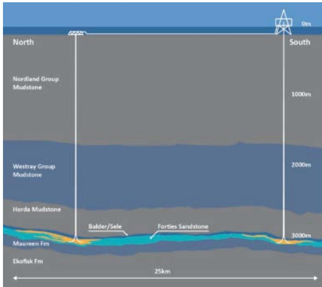
**Figure 28: Forties 5 sandstone aquifer covers over 20,000km<sup>2</sup>. Yellow indicates the potential storage formation. Blue indicates saline fluids. Rig and subsea topsides not to scale (Pale Blue Dot, 2016)**
