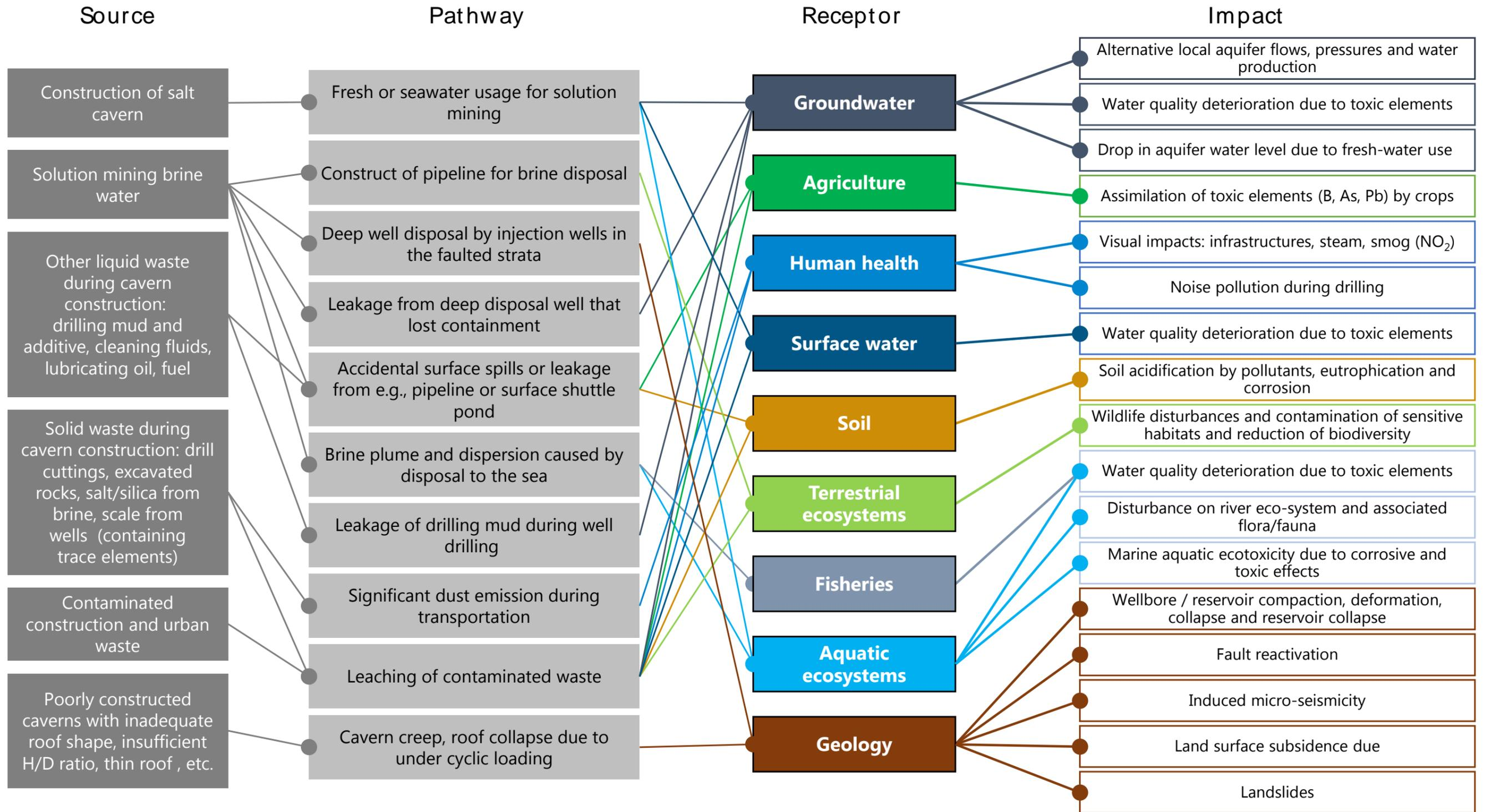
Figure 61: SPR diagram for cavern mining and preparation
