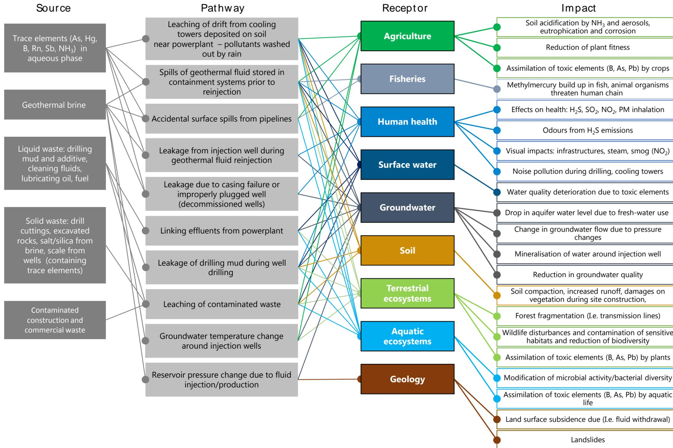
**Figure 55: SPR diagram for hydrothermal systems**
