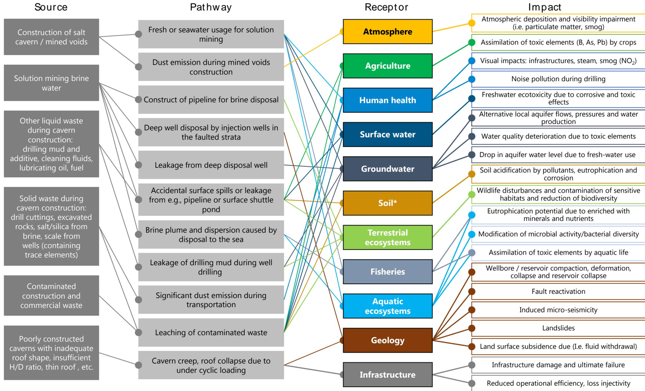
Figure 57: SPR diagram for salt cavern/mined voids for the mining and preparation phase
