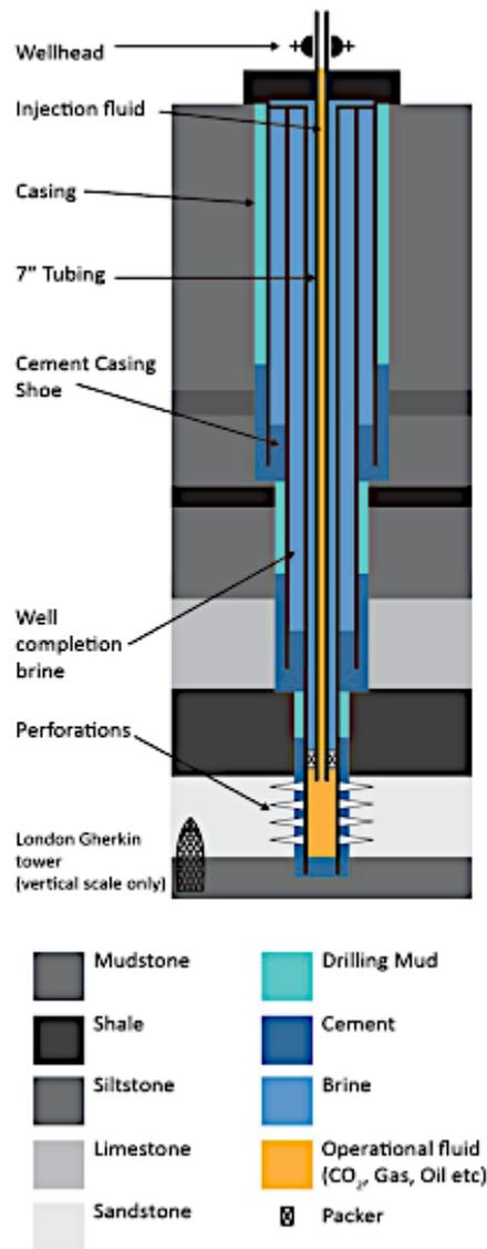
**Figure 22: Schematic of a CCS injection well (Pale Blue Dot, 2016)**
