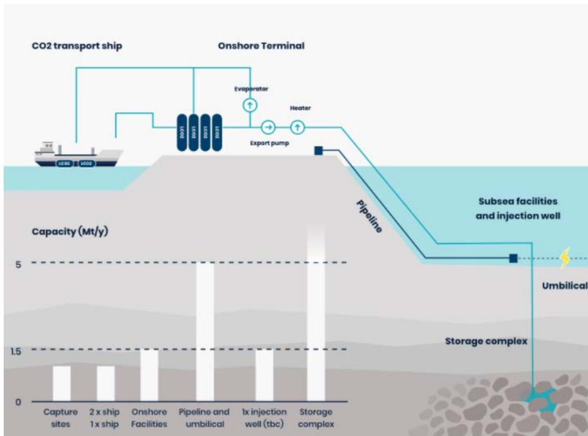
**Figure 21: Overview of Northern Lights CCS project, note intermediate CO<sub>2</sub> storage at onshore terminal (Northern Lights CCS, 2021)**
