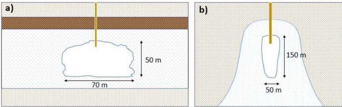
Figure 5: Salt caverns in a) bedded and b) domal salt deposits (Duhan, 2018)
