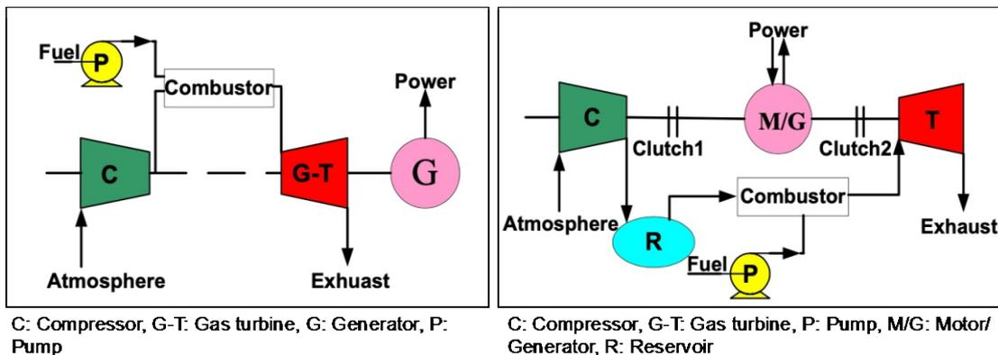
**Figure 7: Left: schematic diagram of gas turbine plant; right: schematic diagram of a CAES plant (Wang and others, 2017)**
