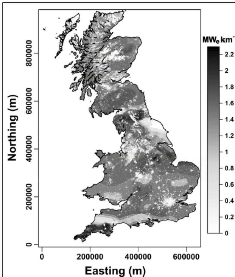
**Figure 36 Technical potential power density across the UK for the depth range of 3,500 to 6,500m. Areas with zero potential are mainly excluded as a result of land cover comprising urban settings and mountains (Busby & Terrington, 2017)**
