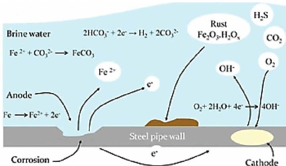
**Figure 24: Illustration of corrosion mechanism for casing steel (Moreno, 2019)**
