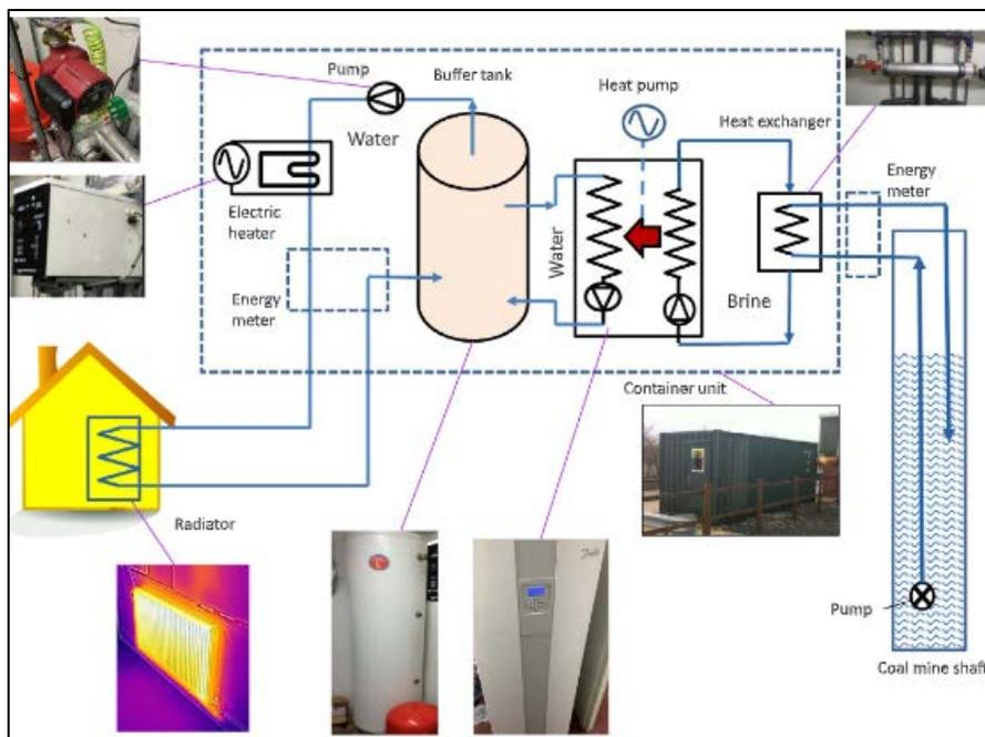
**Figure 31: Schematic of the considered open-loop GSHP system for heating applications from flooded-mine shafts in Markham, UK (Al-Habaibeh and others, 2018)**
