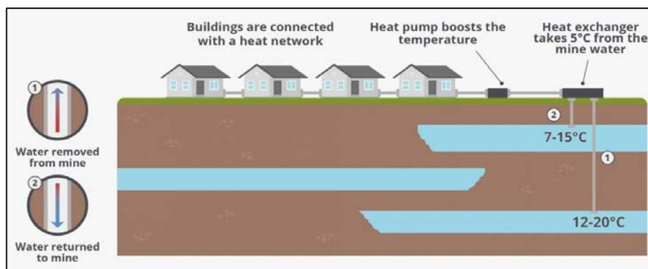
**Figure 32: Infographic demonstrating the potential use of mine water to heat buildings and homes (BGS Press, 2020)**
