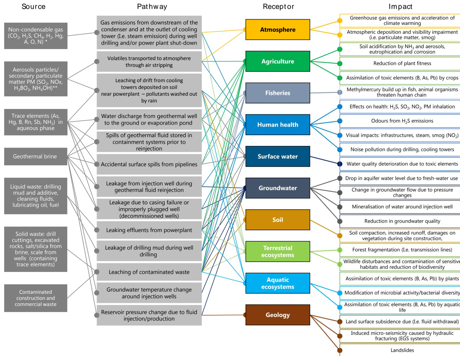
Figure 54: SPR diagram for petrothermal geothermal systems
