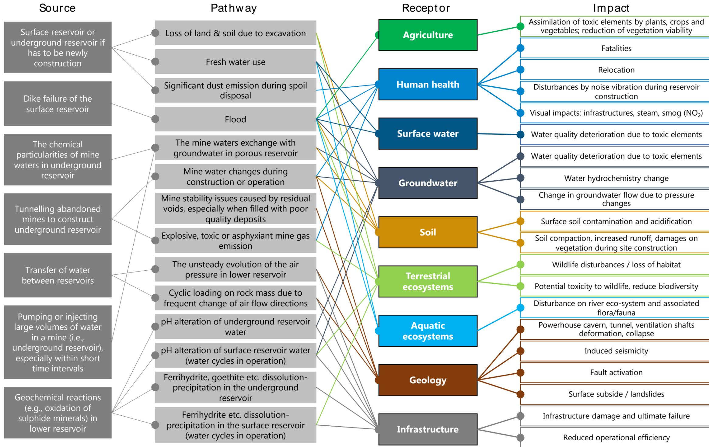
Figure 63: SPR diagram for UPSH operation
