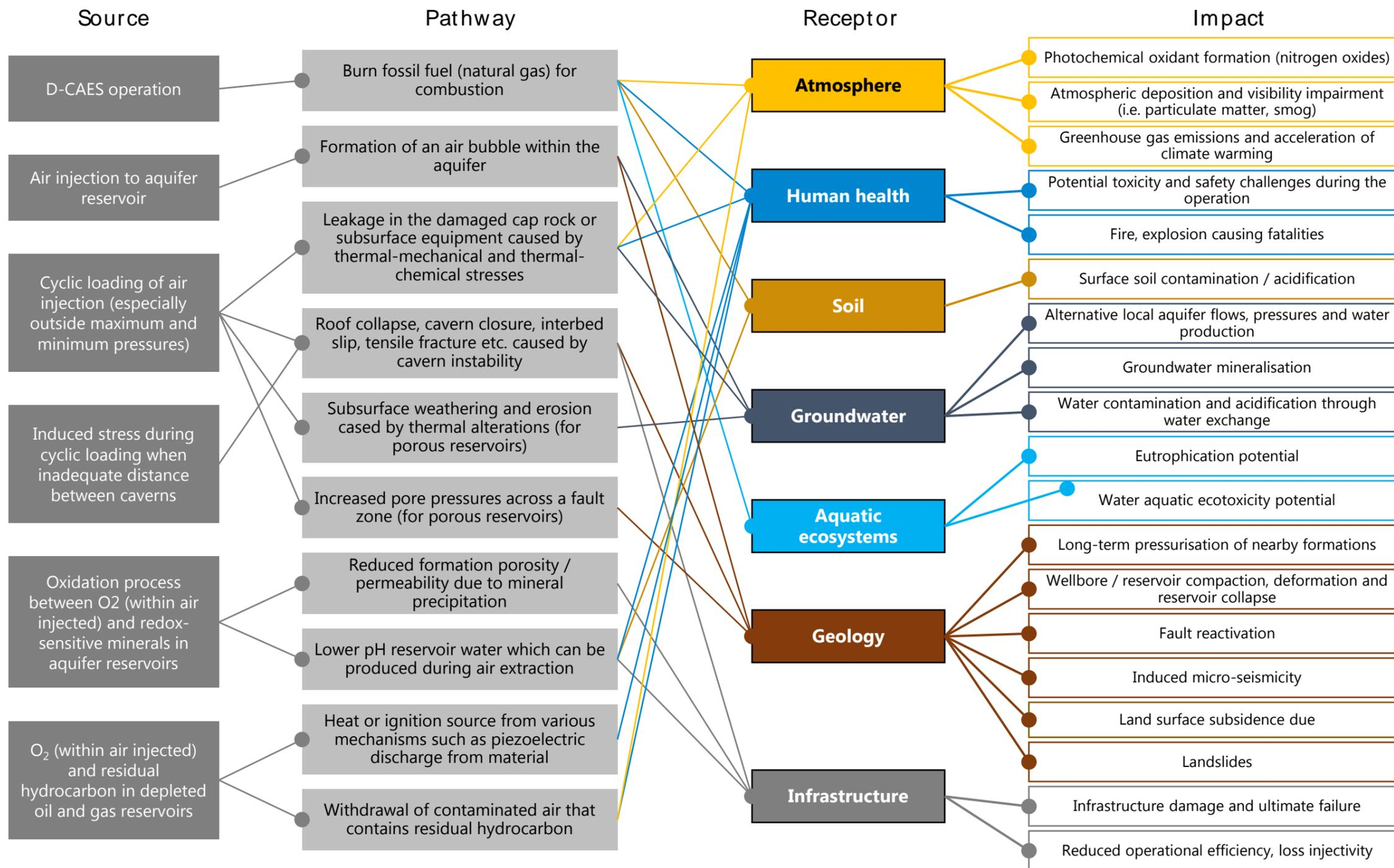
Figure 58: SPR diagram for CAES operations (excluding site preparation)
