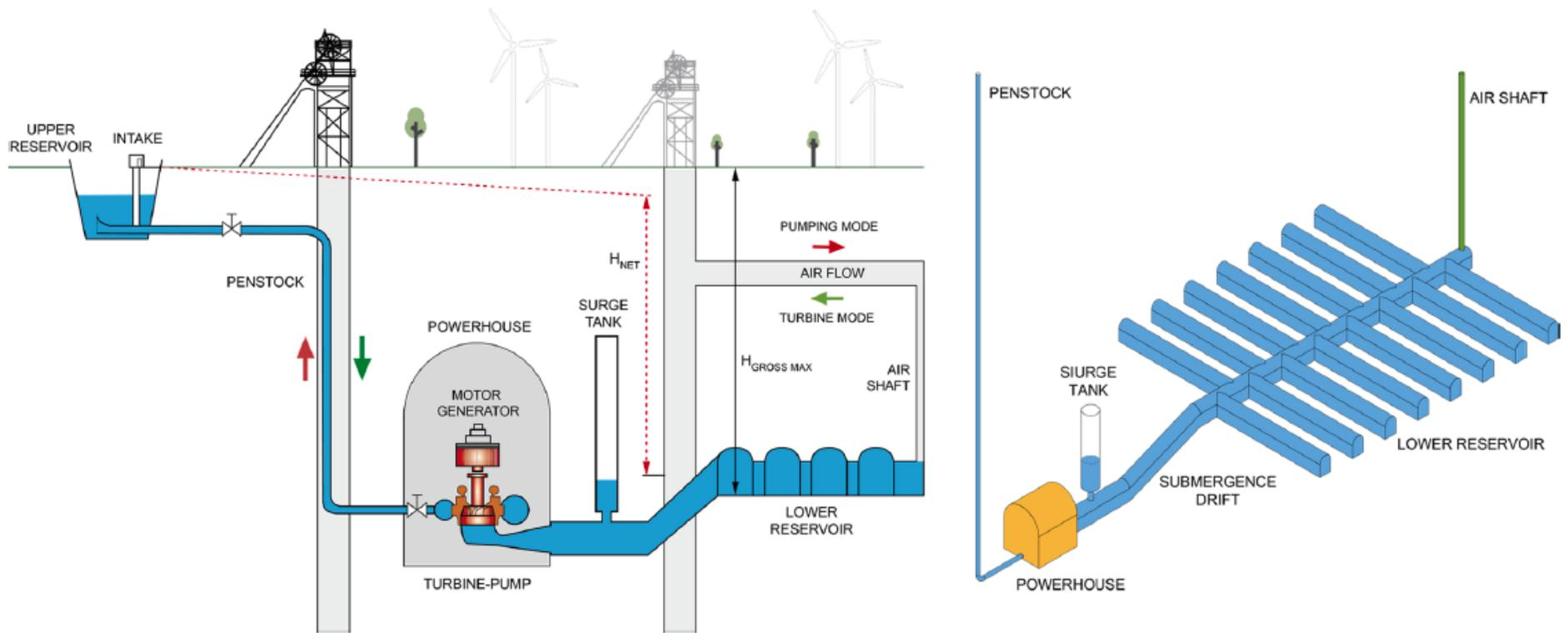
Figure 18: Scheme of UPSH in a closed underground mine: upper and lower reservoir, penstock (for water movement), valve (for flow control), Francis pump-turbine, motor-generator, surge tank and vent shaft (left). 3D detail of the lower reservoir (right) (Menéndez and others, 2019). Gross max head (here  $H_{gross\ max}$ ) shows the maximum potential energy of the system. The larger the maximum head, the more energy can be generated (or consumed to pump to the upper reservoir).
