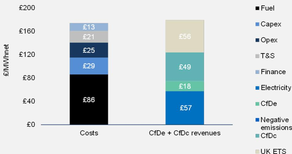
**Figure B2: Levelised costs and revenues for the CfDe + CfDc framework<sup>B5</sup>**
