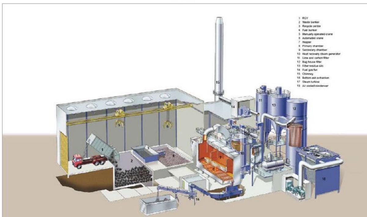
**Figure 34: Schematic of the Energos gasification system**
