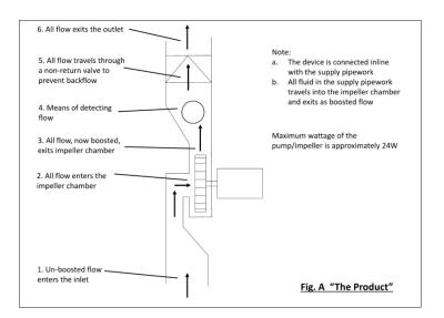
23. In use, all fluid that enters the fluid inlet sequentially flows through the impeller chamber, the non-return valve, and to the outlet in a single unbranched route.
