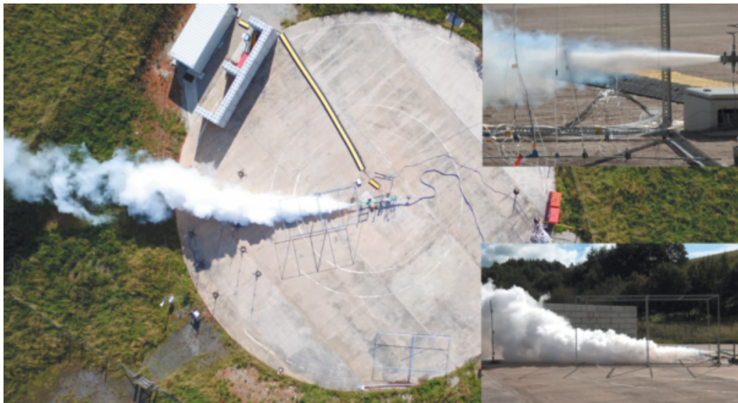
Overhead and close-up images of an elevated liquid hydrogen release at the Frith Valley test site, Buxton
