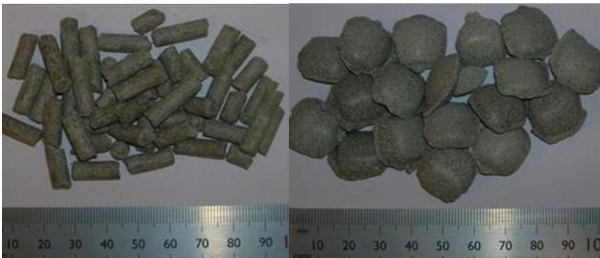
***Figure 3-4 Pictures of the two pellets types used in the erosion tests in the Eva-project. Extruded rod-shaped pellets to the left and roller compacted pillow shaped to the right.***
