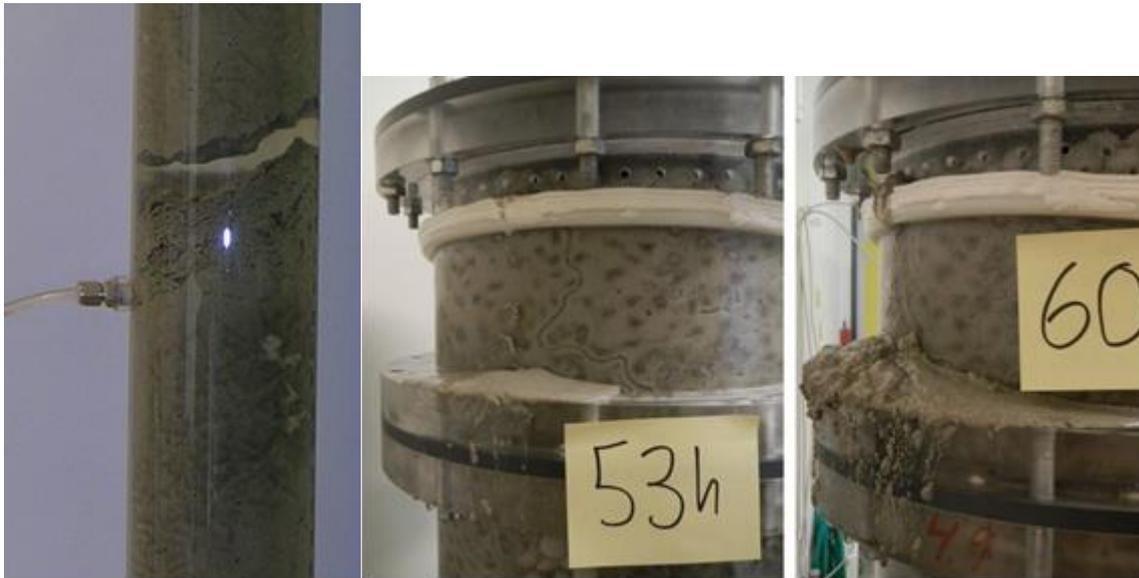
**Figure 3-9** Examples of pocket formation (left) and gel extrusion (Börgesson et al., 2015).
