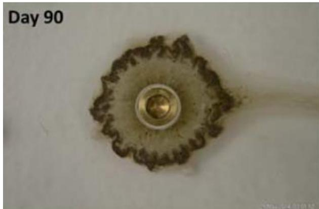
**Figure 4-25** Top view of bentonite extrusion into the fracture after 90 days. The ring of accessory minerals is clearly visible outside the MX-80 bentonite. From Reid et al. (2015).
