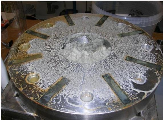
*Figure 3-8 Distribution of bentonite in the fracture after removal of the upper part in test 12 (aperture 0.05 mm, flow rate 0.1 l/min and pressure increase rate 2 MPa/h). The pellet-filled cylinder is seen in the centre. The strips are placed for fixing the slot width.*
