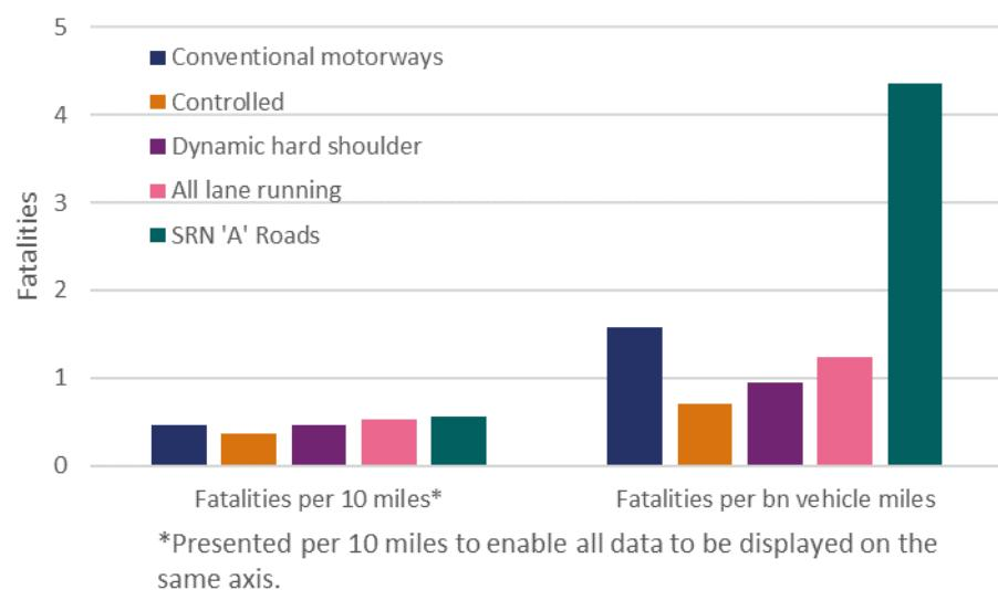
This shows that fatality rates per mile are similar on SRN 'A' roads and motorways. However, fatality rates per vehicle mile are much higher on SRN 'A' roads in comparison to motorways. The reason for this is that motorways carry significantly more traffic per mile than SRN 'A' roads, which results in comparatively lower fatality rates per vehicle mile travelled.
