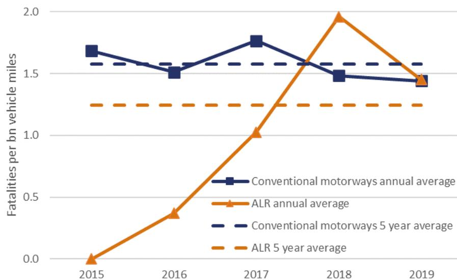
**Figure A.7: Comparison of annual and three-year average fatality rates per bn vehicle miles for conventional and ALR motorways**
