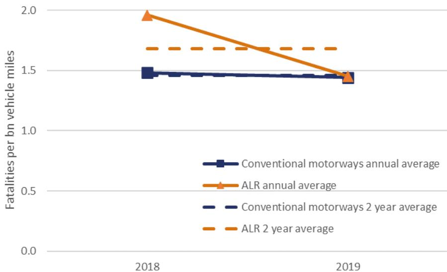
**ORR assessment:** Total vehicle miles driven on ALR motorways in 2015 is small (1.4bn vehicle miles) compared to 2019 (6.2bn vehicle miles). The averages in the *Smart Motorway Safety Evidence Stocktake and Action Plan* and *First year progress report* are weighted by traffic volume to account for this.
