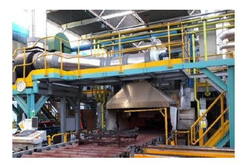
The entrance to the WS2 sag-bend furnace located at the Lathom site
