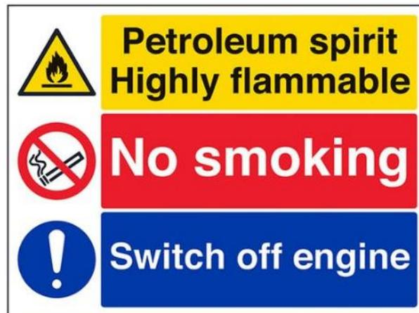
Figure 7 – Typical Sign at Dispensers and Tank Fill Points.
