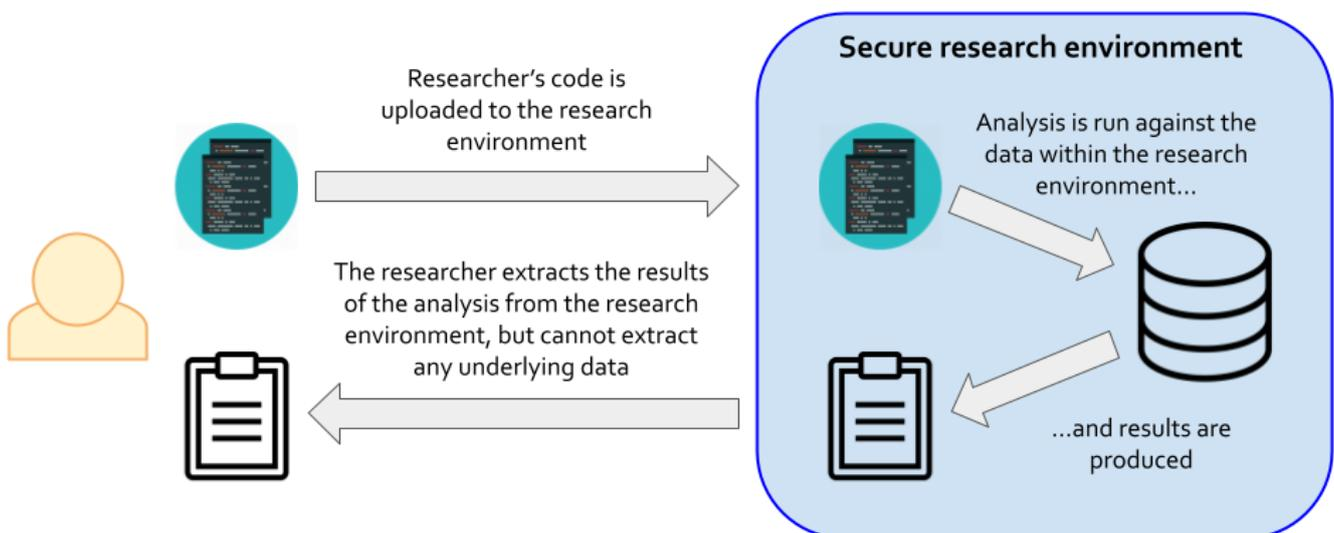
**Exhibit 2** shows a high-level overview of a data custodian that manages a secure research environment holding highly sensitive data, such as healthcare data. In this example, a researcher uploads their analytic code to the environment where it is executed against the data. The researcher is unable to copy or extract any of the raw data from the environment, only the results of the analysis.
