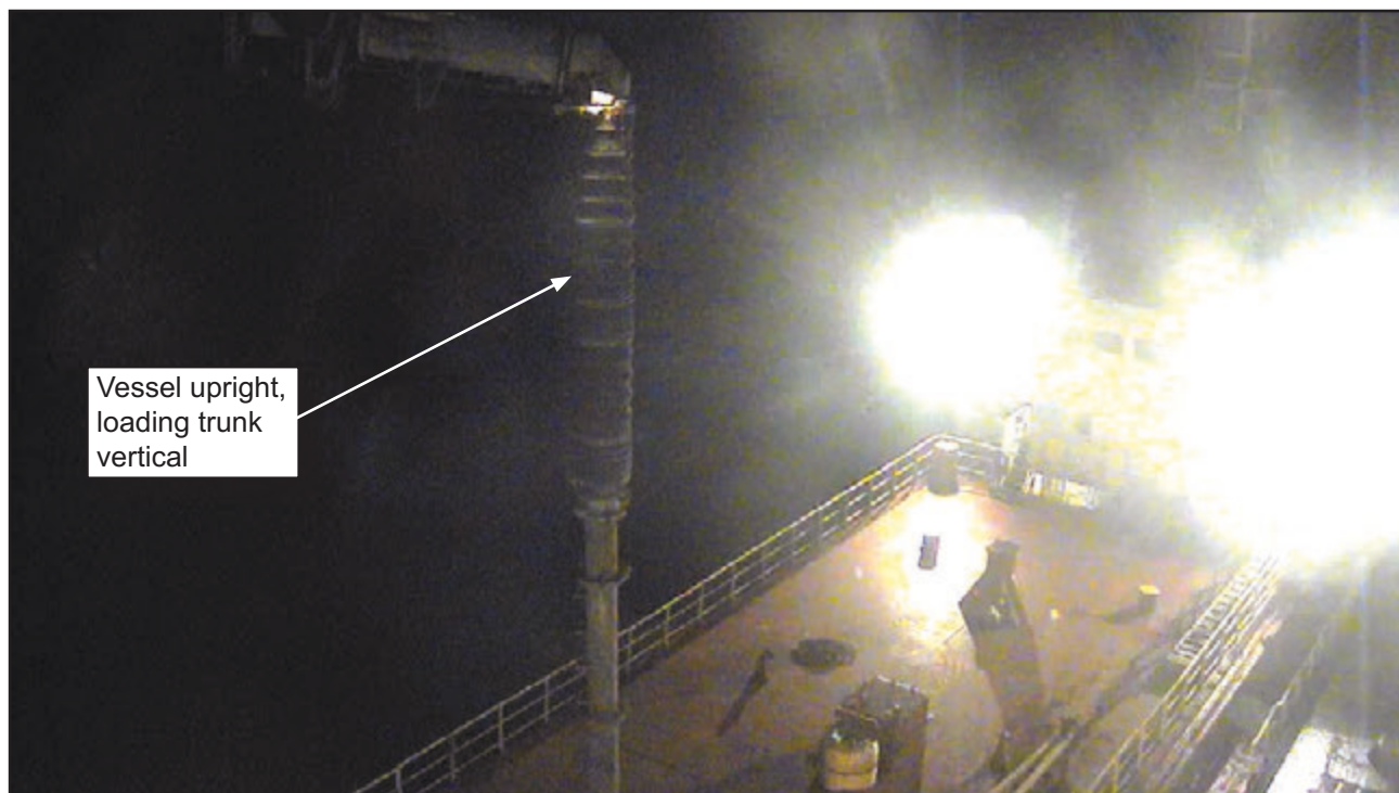
Figure 1a: CCTV image of Cemfjord alongside in Rordal at 0119, 30 December 2014. Vessel is upright, cement loading trunk is vertical
