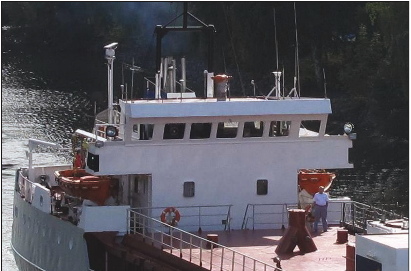
Figure 50: Cemfjord - original open lifeboat installation
