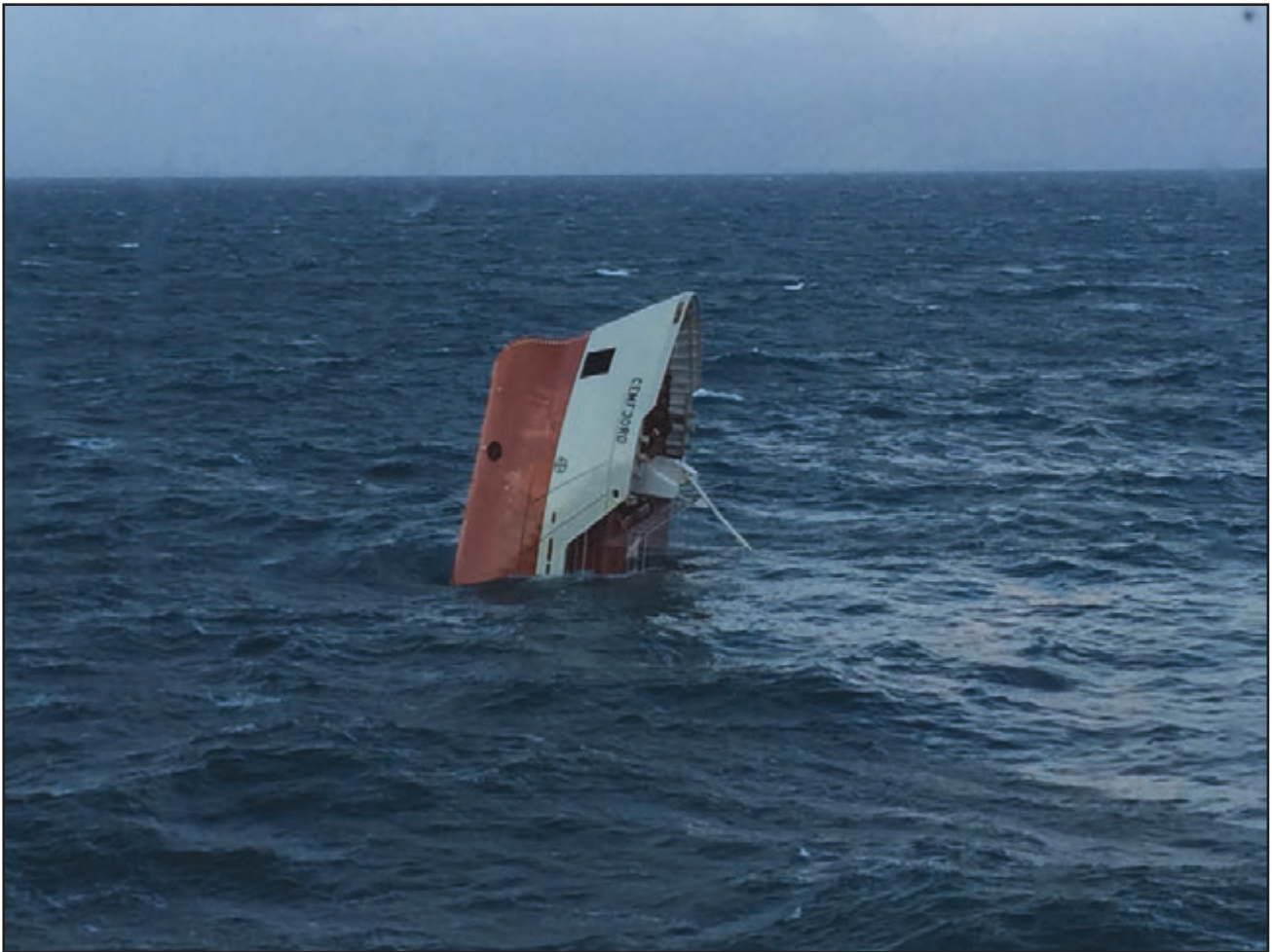
Figure 9: Cemfjord's hull after moving to a vertical position
