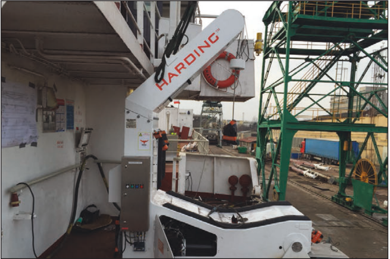
Figure 51: Replacement Harding davit (starboard side)
