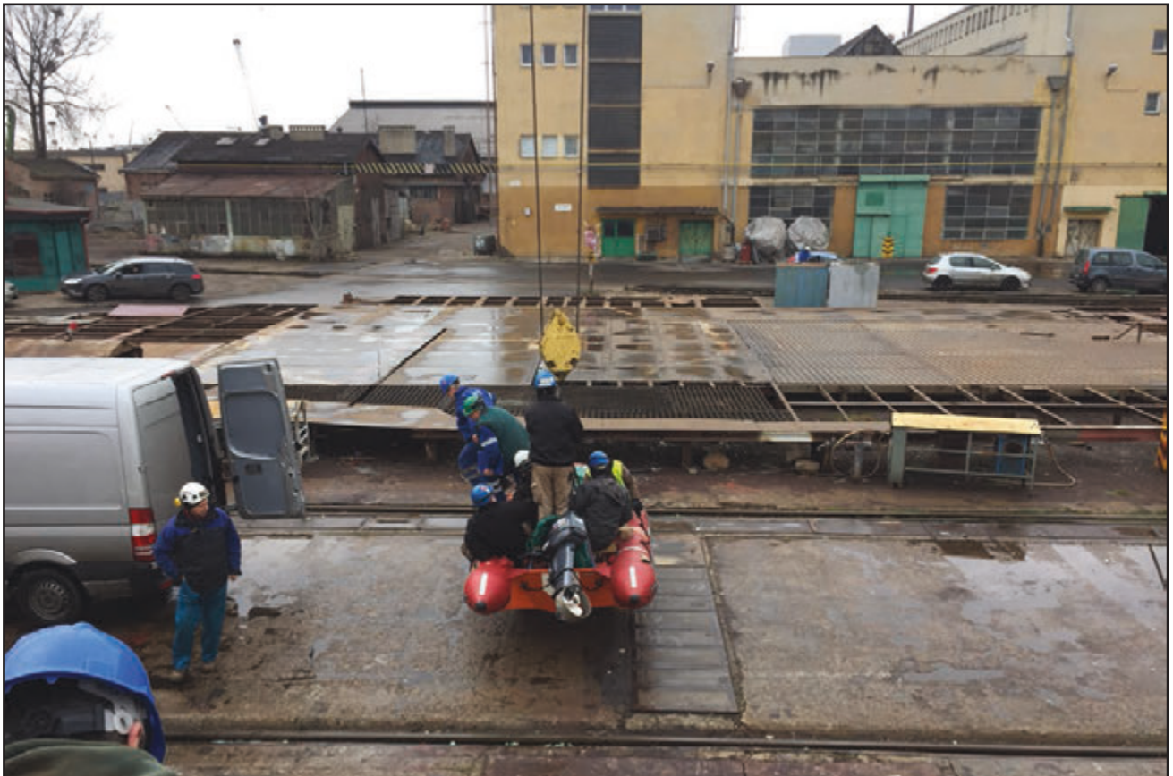
Figure 52: Temporary rescue boat load test with seven persons embarked during refit period in Poland
