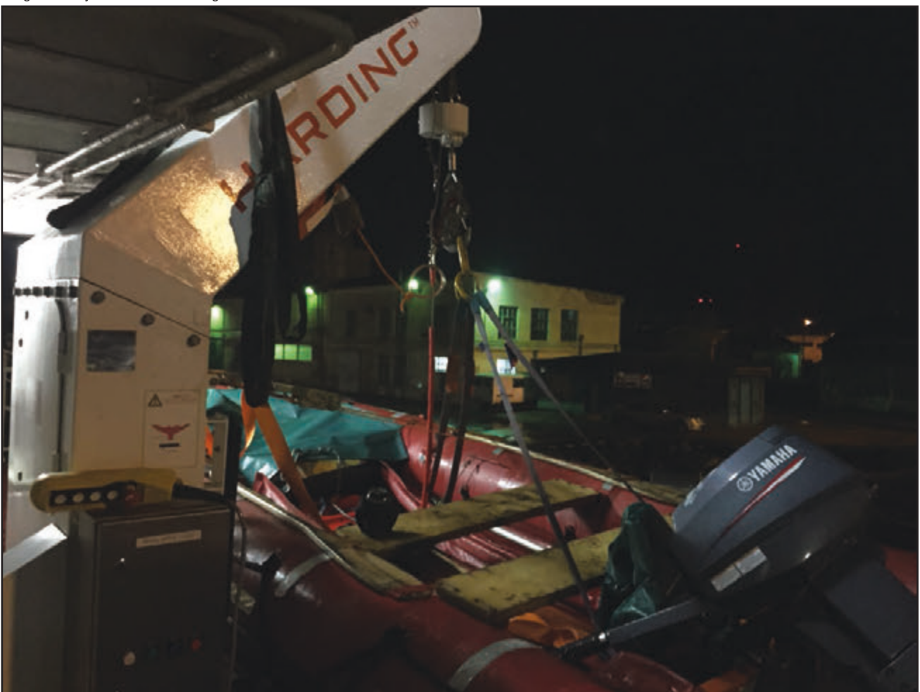
Figure 21: Zodiac temporary rescue boat in replacement Harding davit
