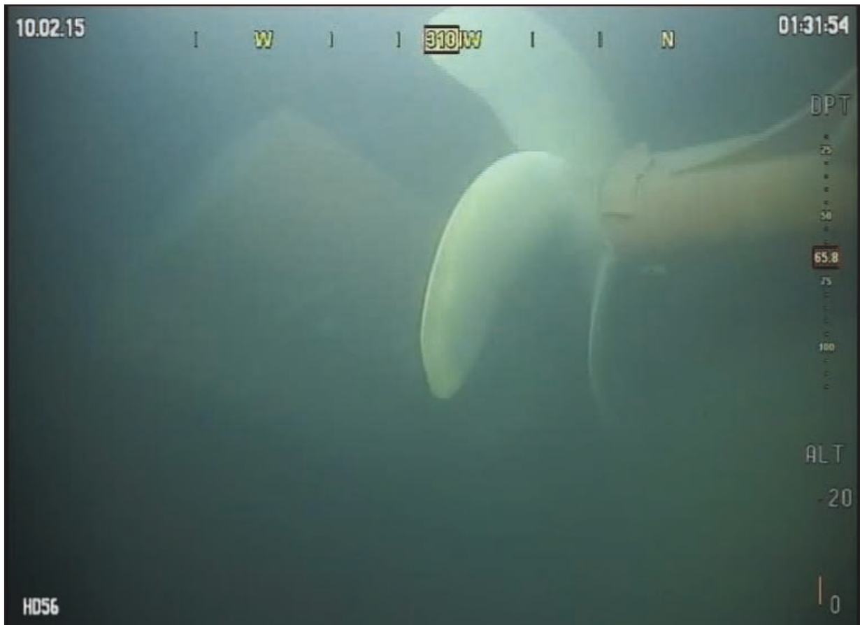
Figure 34: Wreck of Cemfjord - propeller with rudder set to approximately 10° to port
