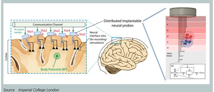
Schematic of the 'Neurograins' system, which intends to establish a 'cortical intranet' of multiple implants
