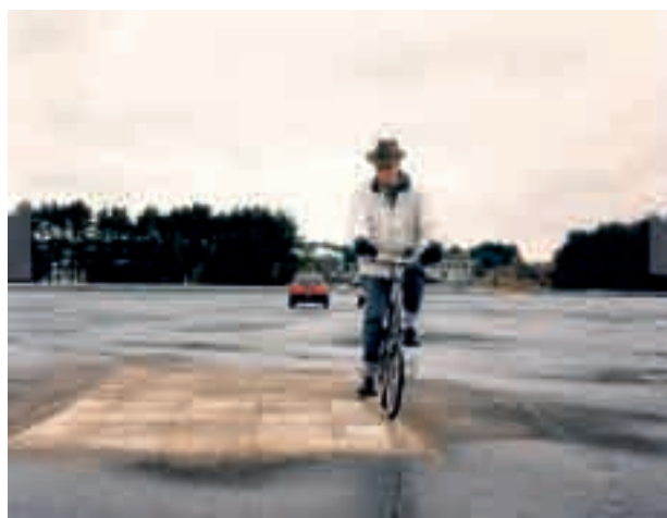
Fig. 2.7 Cyclist involved in track trials of humps
